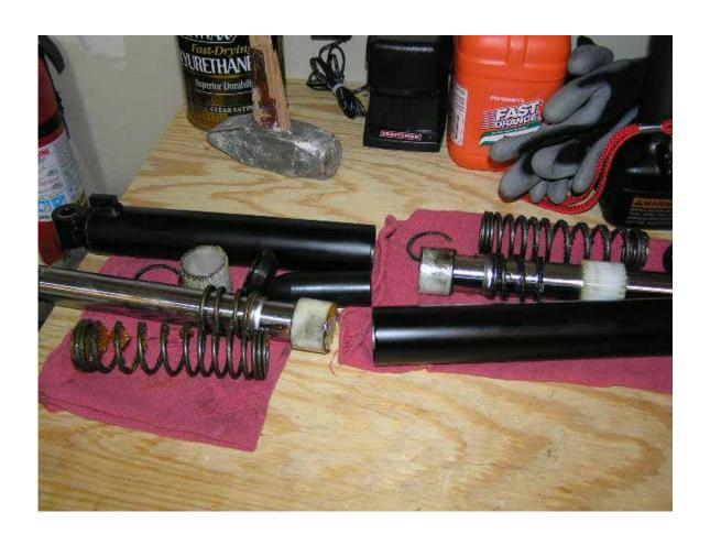
Now that you have the forks apart take the rubber stopper and cut two 1 inch pieces from it. Being very careful to accurately measure each piece and cut through squarely. I used a ratcheting PVC cutter for this. A Craftsman Handi-cut will work or even a Utility knife just be sure to make your cuts as square as possible. You will have the cone shaped end piece left over and can discard it if you like.
