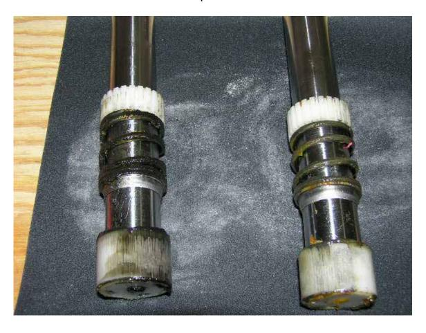
Putting the springs and rubber bumper in the proper order and assembling will look like this. From the left in order: Added Rebound spring, Die spring, rubber bumper, and main spring. When assembled they look like the 2<sup>nd</sup> picture.
