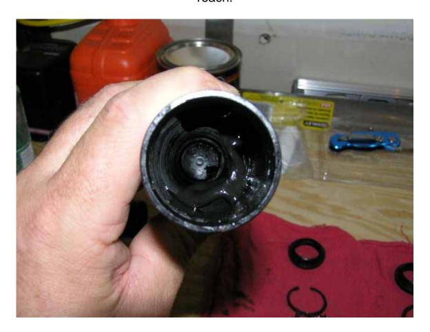
You can now install the spring assembly. (*Insert added rebound, die spring, and rubber end toward the bottom of fork and with the tapered end of the main spring at the top*)
