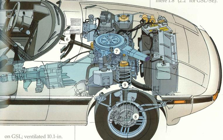
on GSL; ventilated 10.1-in. rear discs standard on GSL-SE, for maximum faderesistant high performance. Parking brake mechanically activated on rear wheels.
