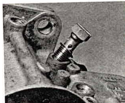
5.11 Removing a main jet holder
