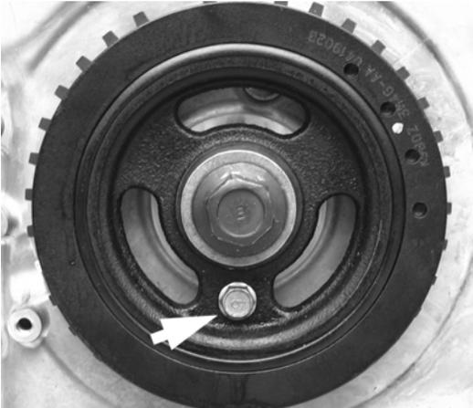
21. Remove the crankshaft timing peg 303-507.
