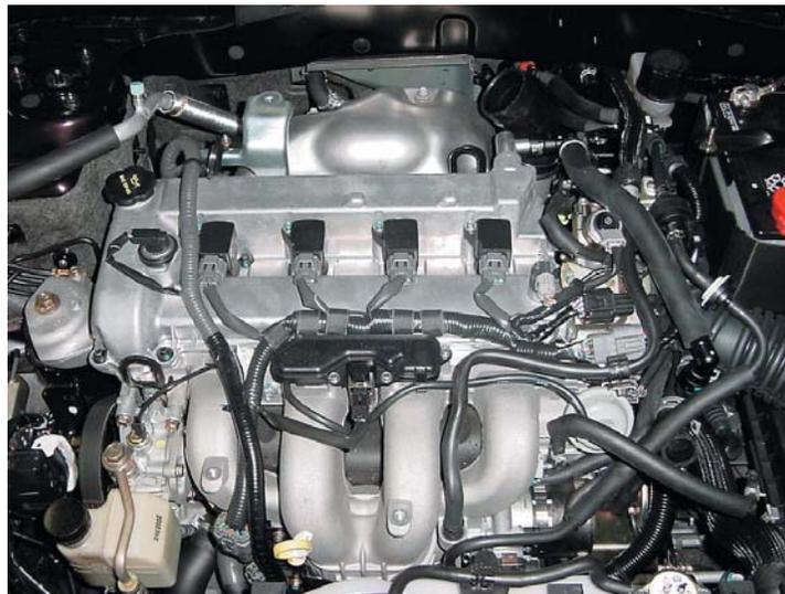
5. MX-5 Miata: remove the fresh air box and the battery to access the front of the engine.
