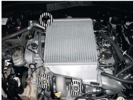
C. Remove the air bypass control hose clamp and disconnect the hose from the valve.
