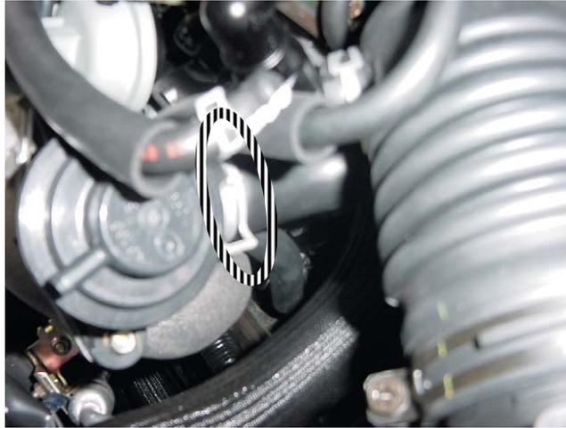
E. Loosen the hose clamp from the turbo outlet to the intercooler inlet (10mm or #2 Phillips).
