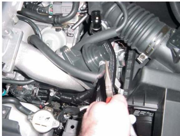
D. Loosen the bypass outlet hose clamp.
