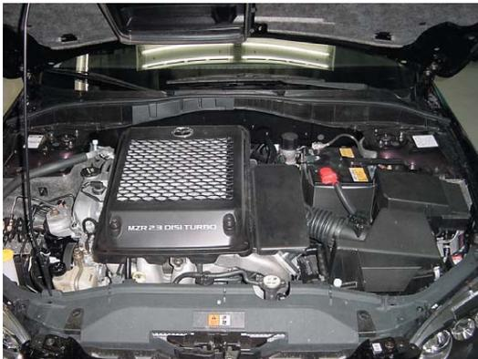
A. CX-7: remove the two plastic clips securing the intercooler shroud to the vehicle and remove the three 10mm bolts securing the plastic intercooler cover.
