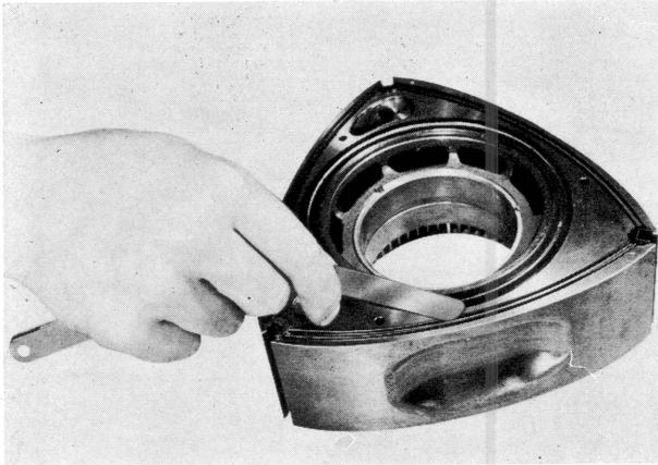
Fig. 1-72 Checking side seal gap
