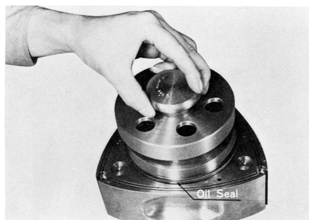
Fig. 1-85 Installing outer oil seal
