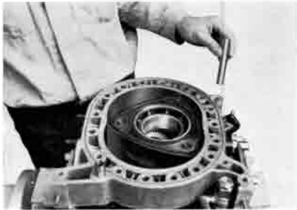
Fig. 1-96 Installing tubular dowels
