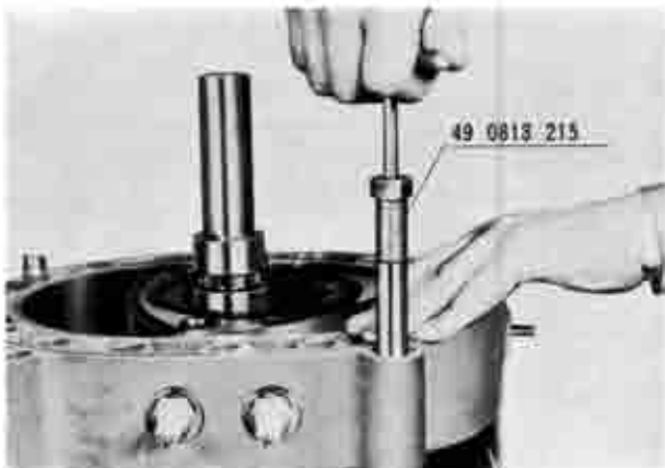
Fig. 1-26 Pulling tubular dowels
