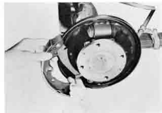
Fig. 10-24 Installing operating strut
