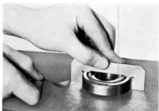
Fig. 9-18 Checking bearing model height
