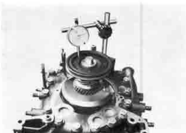
Fig. 1-104 Checking end play
