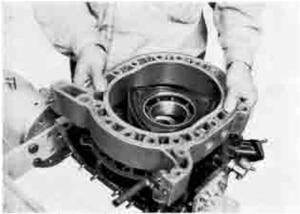
Fig. 1-95 Installing rear rotor housing
