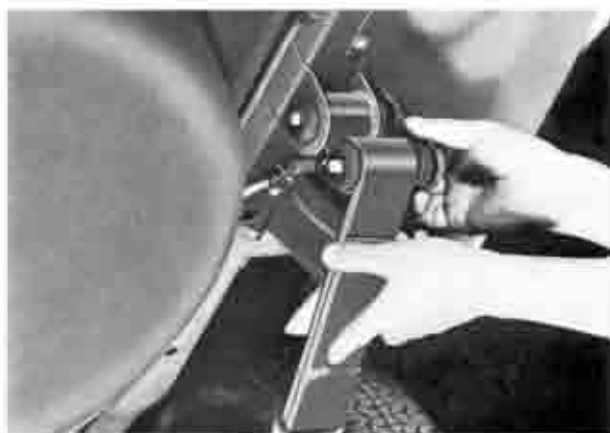
Fig. 13-26 Installing rear side of the rear spring
