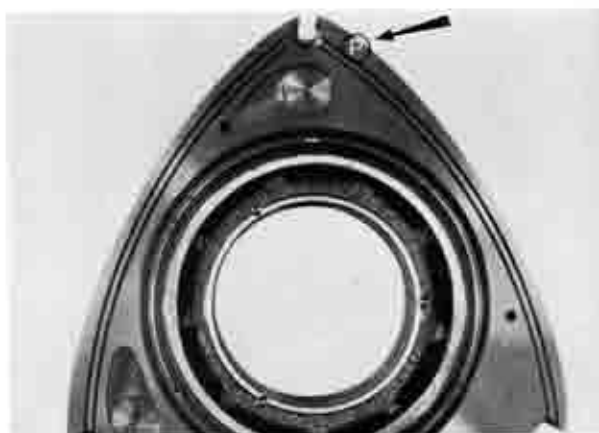
Fig. 1-76 Mark of corner seal groove
