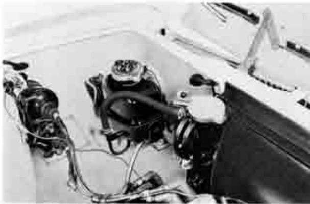
Fig. 3-2 Radiator and expansion chamber
