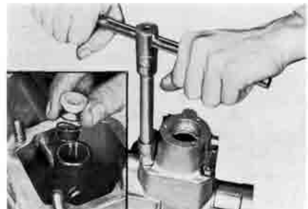
Fig. 7-20 Installing control case
