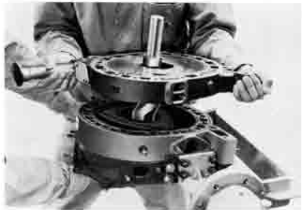
Fig. 1-100 Installing intermediate housing
