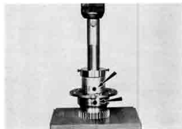
Fig. 1-42 Installing main bearing
