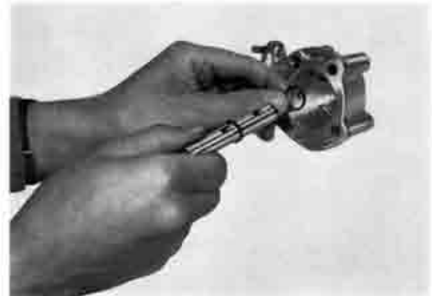
Fig. 2-8 Assembling oil pump
