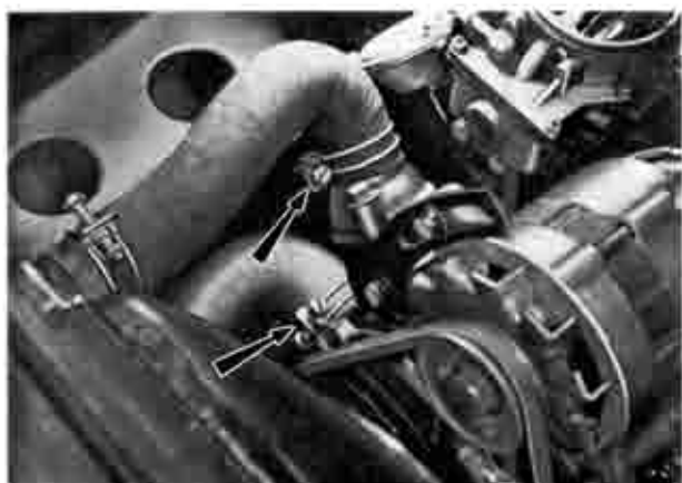
Fig. 1-8 Removing water hoses
