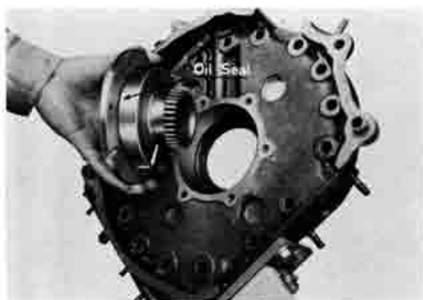
Fig. 1-46 Installing stationary gear
