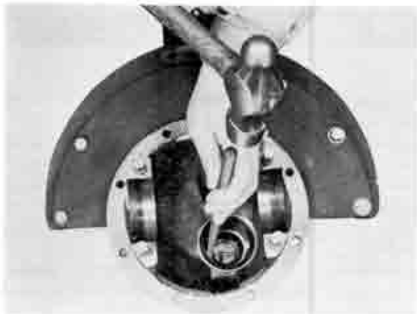
Fig. 9-10 Removing bearing outer race
