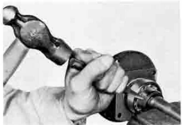
Fig. 9-3 Cutting bearing collar
