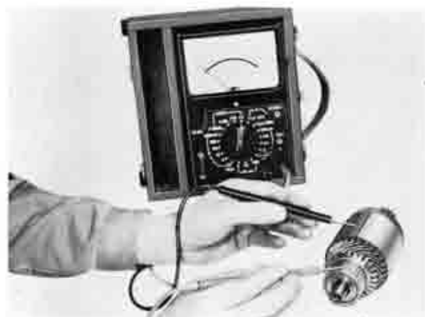
Fig. 5-26 Checking armature for ground
