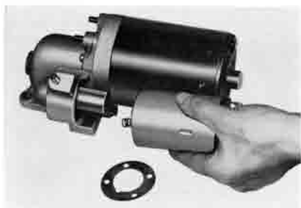
Fig. 5-22 Removing magnet switch
