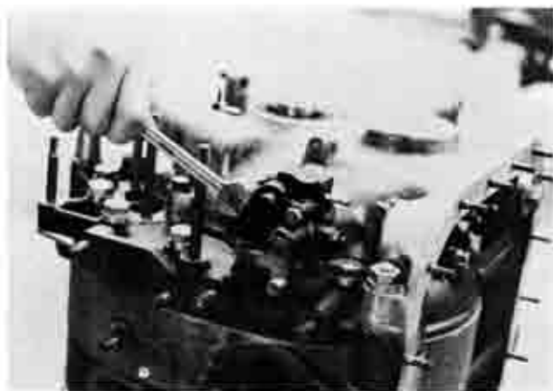
Fig. 1-21 Removing metering pump
