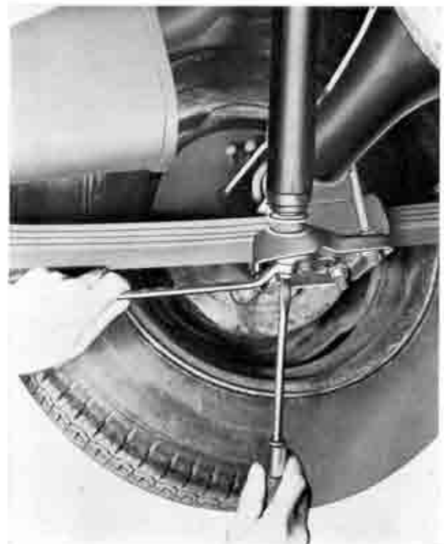
Fig. 13-23 Installing shock absorber
