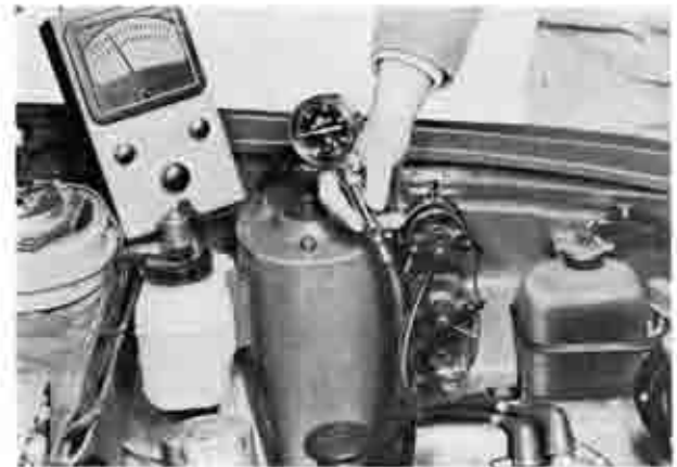
Fig. 2-4 Checking oil pressure
