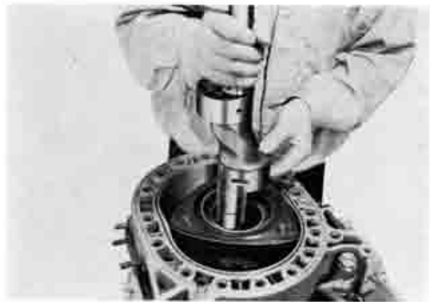
Fig. 1-99 Installing eccentric shaft
