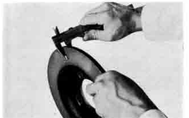
Fig. 10-21 Checking disk thickness
