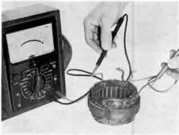
Fig. 5-12 Checking stator coil for open.
