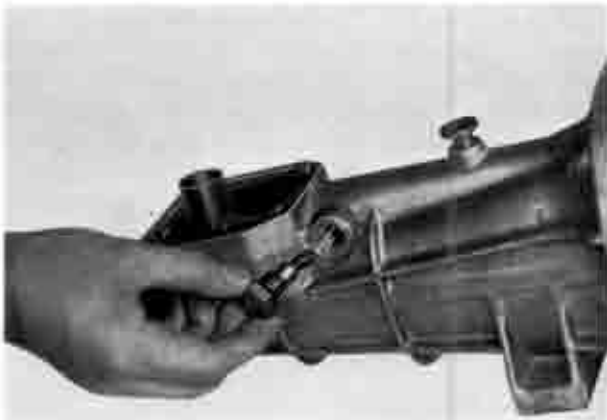
Fig. 7-17 Installing friction piece
