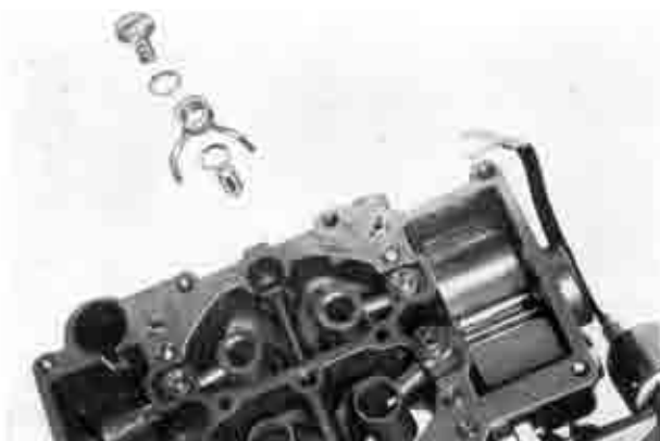
Fig. 4-8 Removing pump nozzle
