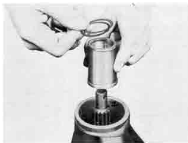
Fig. 9-19 Installing spacer and shim
