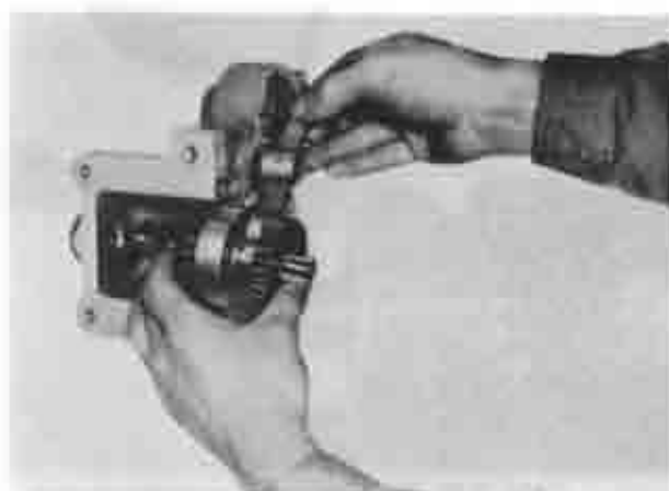
Fig. 5-25 Removing driving lever
