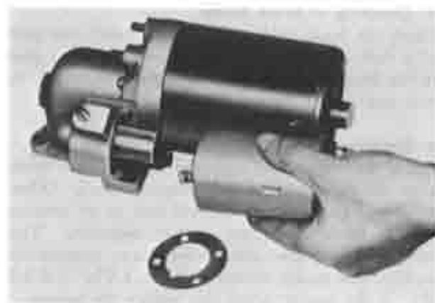
Fig. 5-22 Removing magnet switch
