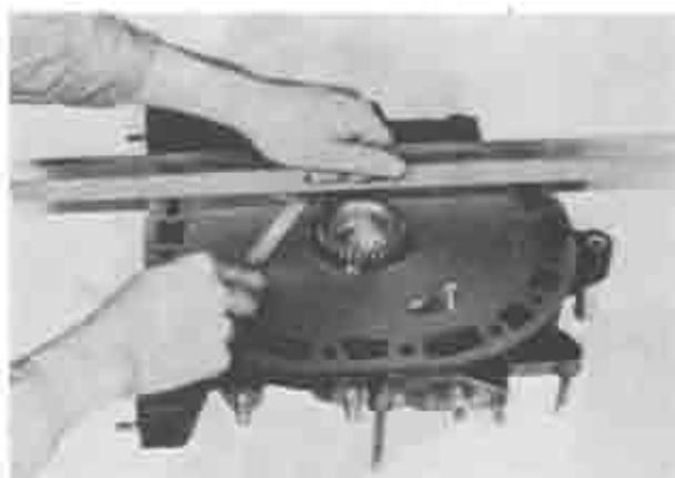
Fig. 1-35 Checking front housing distortion
