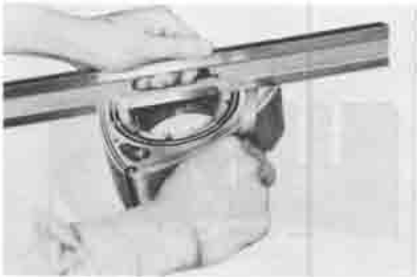
Fig. 1-56 Inspecting land protrusion
