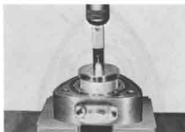
Fig. 1-60 Installing rotor bearing
