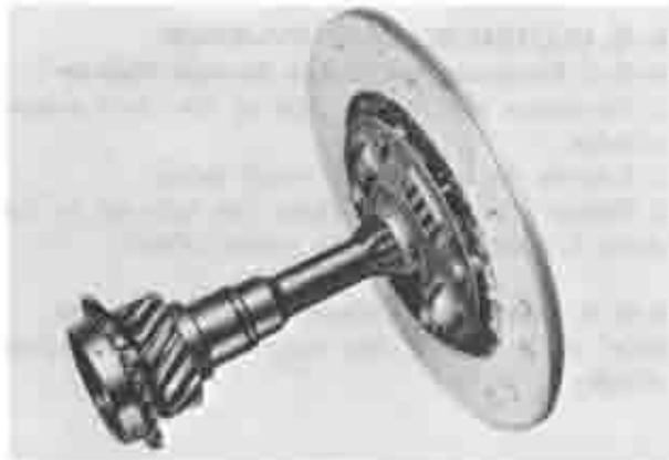
Fig. 6-5 Checking spline fit of clutch disk
