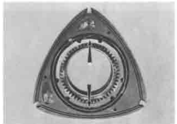
Fig. 1-84 Position of spring gap
