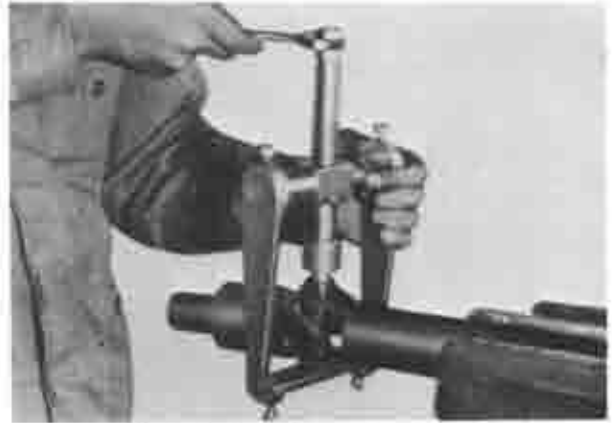
Fig. 8-7. Assembling universal joint.
