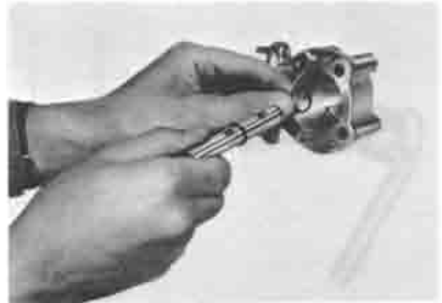
Fig. 2-8 Assembling oil pump
