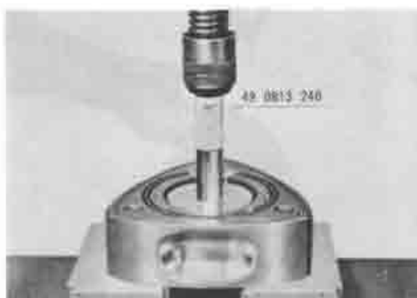
Fig. 1-59 Removing rotor bearing
