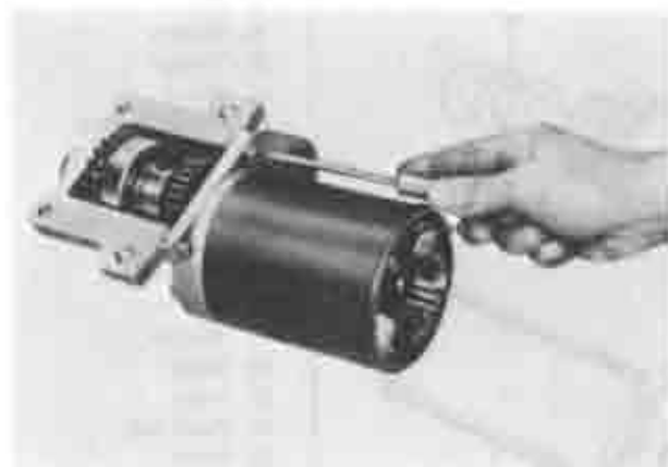
Fig. 5-24 Removing field coil
