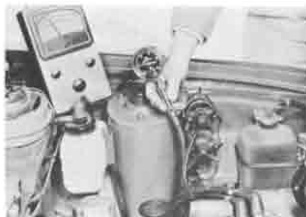
Fig. 2-4 Checking oil pressure
