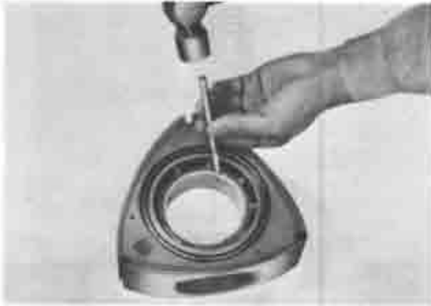
Fig. 1-63 Staking locking screws
