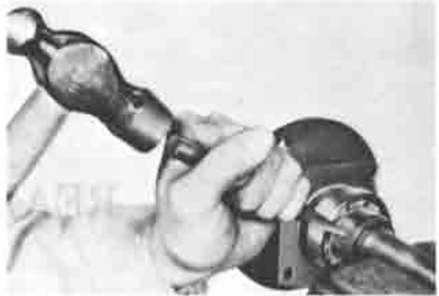
Fig. 9-3 Cutting bearing collar
