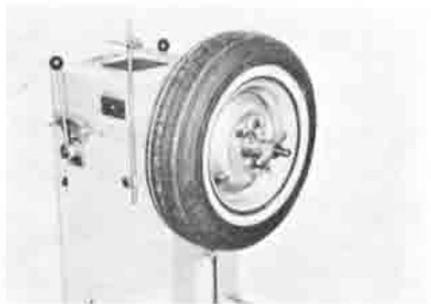
Fig. 12-2 Checking wheel balance
