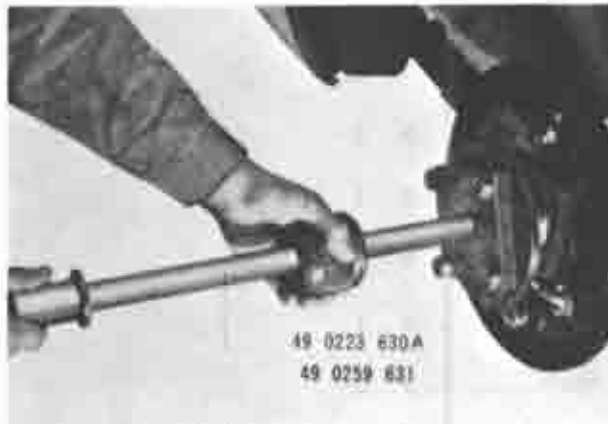
Fig. 9-1 Extracting rear axle shaft.
