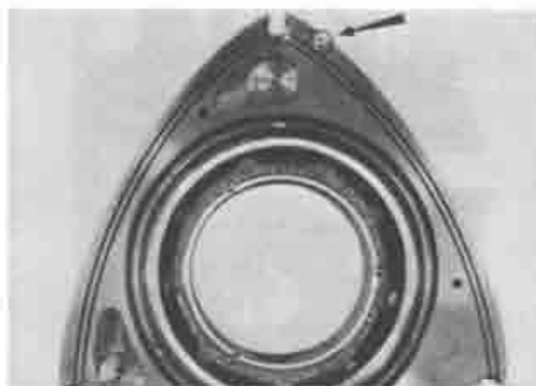
Fig. 1-76 Mark of corner seal groove
