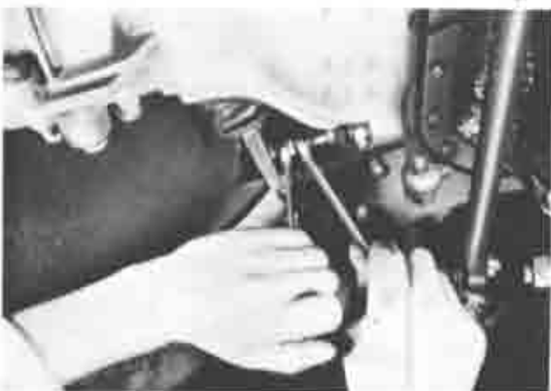
Fig. 6-2 Adjusting the release fork
