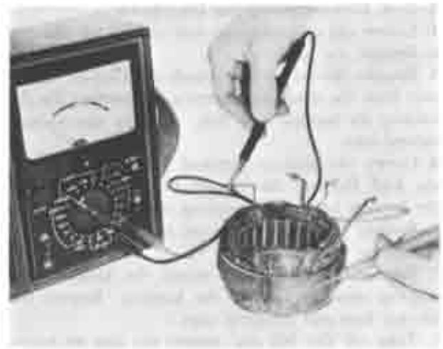
Fig. 5-13 Checking stator coil for ground
