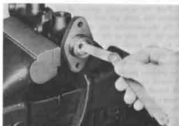
Fig. 10-6 Checking piston clearance
