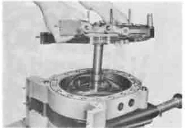
Fig. 1-101 Installing front housing
