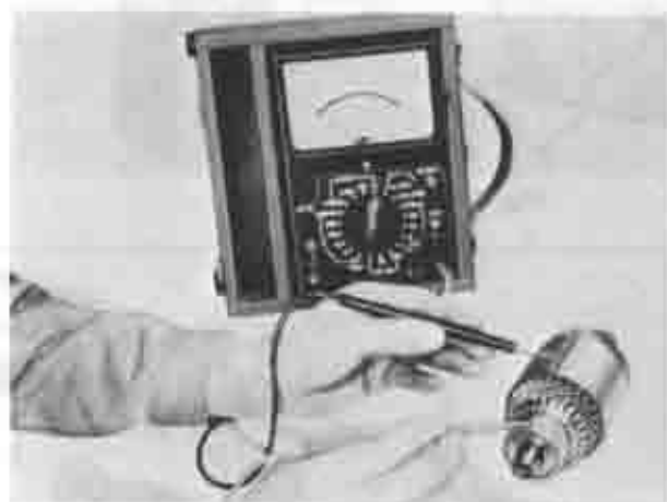
Fig. 5-26 Checking armature for ground
