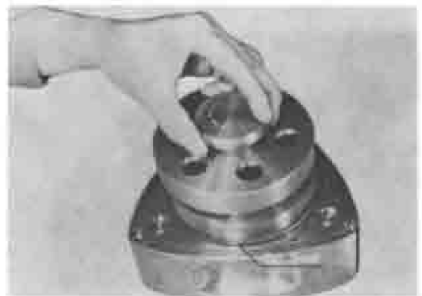
Fig. 1-85 Installing outer oil seal
