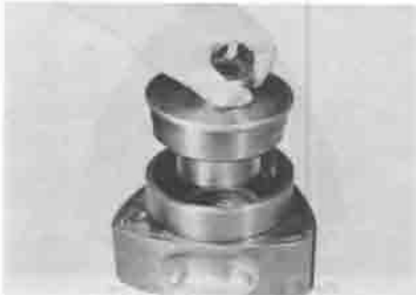
Fig. 1-88 Installing inner oil seal
