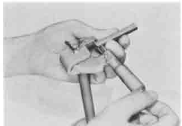
Fig. 1-68 Measuring apex seal height
