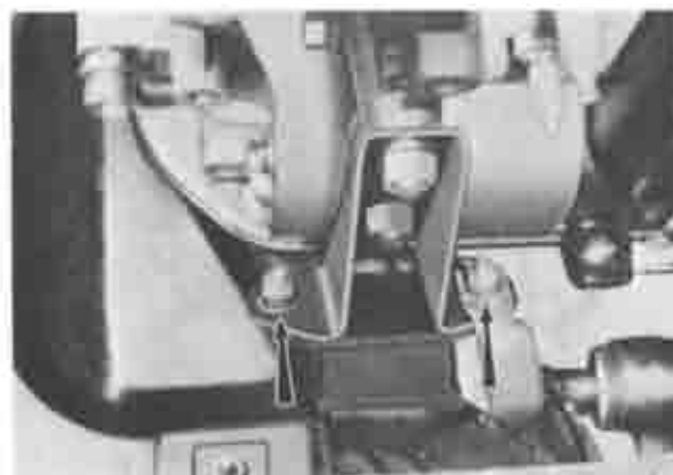
Fig. 1-12 Loosening mounting bolts
