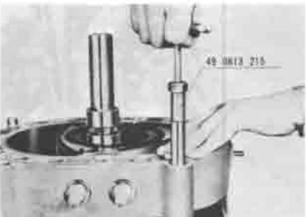
Fig. 1-26 Pulling tubular dowels
