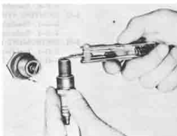
Fig. 5-2 Checking spark plug gap
