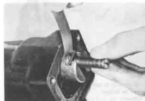
Fig. 11-6 Checking end clearance
