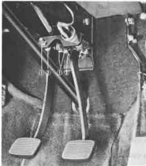
Fig. 6-1 Clutch pedal adjustment
