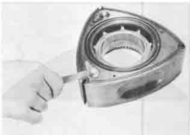
Fig. 1-74 Checking corner seal gap
