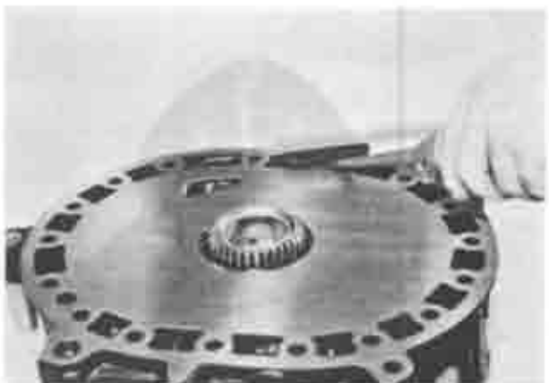
Fig. 1-34 Cleaning front housing
