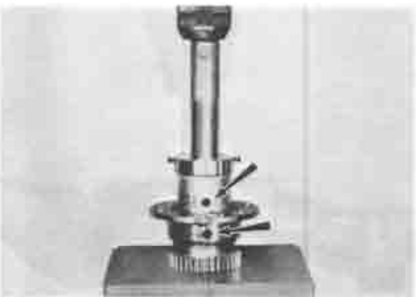
Fig. 1-42 Installing main bearing
