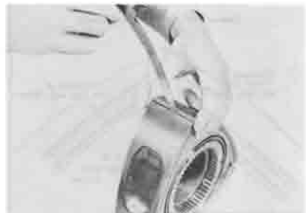
Fig. 1-69 Checking gap of apex seal and groove
