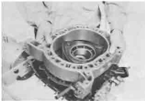
Fig. 1-95 Installing rear rotor housing
