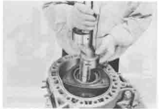
Fig. 1-99 Installing eccentric shaft
