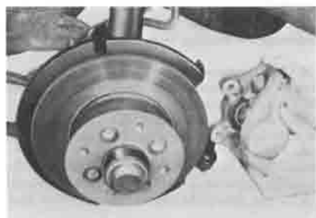
Fig. 10-13 Lifting off caliper
