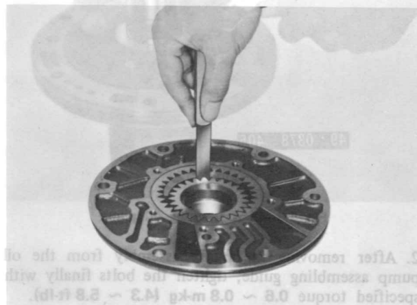
Fig. 7B-41 Measuring clearance (2)
