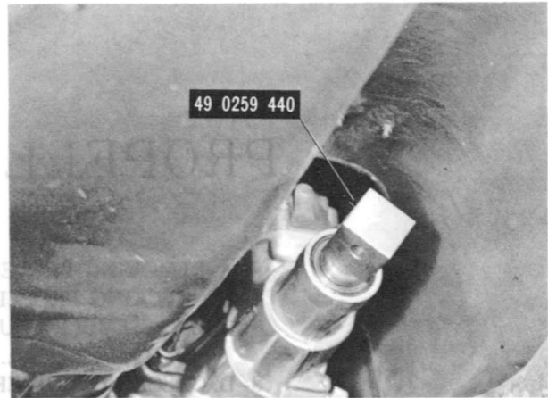
Fig. 8-1 Holder installed into extension housing
