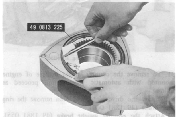
Fig. 1-24 Removing oil seal
