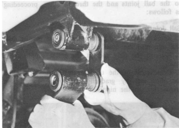
Fig. 13-11 Installing shackle pin
