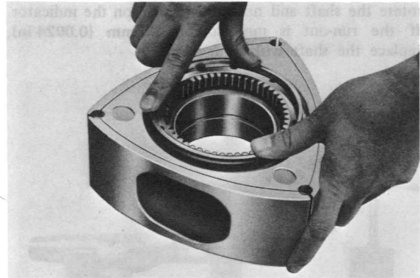
Fig. 1-64 Installing oil seal
