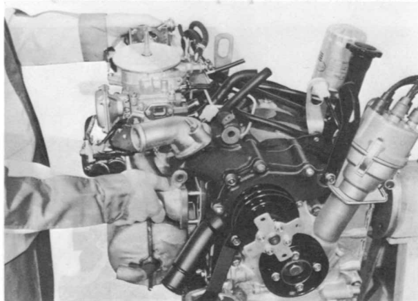
Fig. 1-5 Removing intake manifold ass'y
