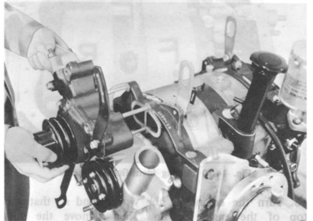
Fig. 1-7 Removing water pump
