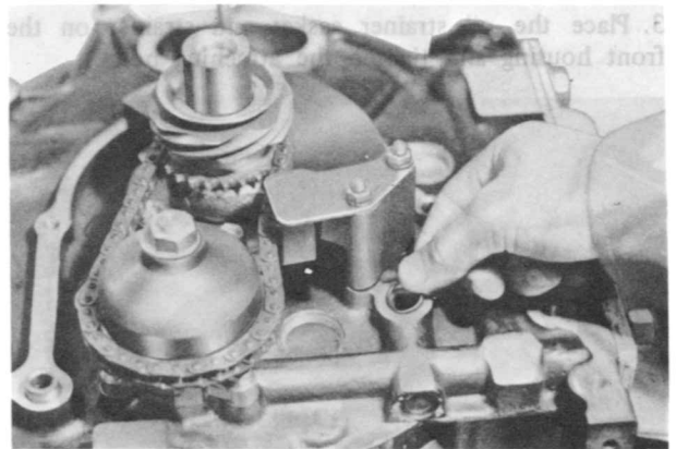
Fig. 1-87 Placing "O" ring
