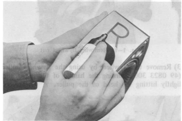
Fig. 1-23 Putting identification mark
