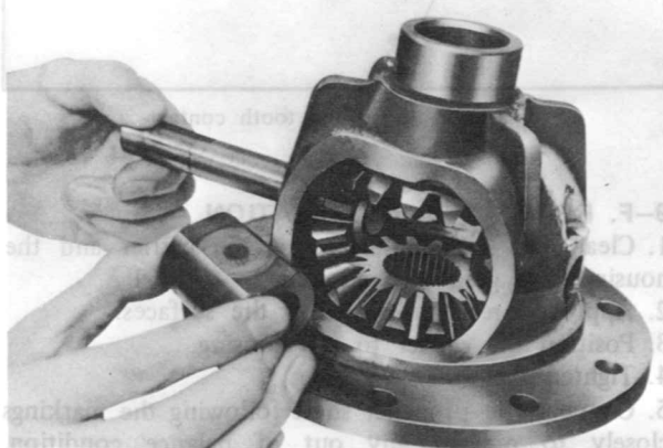
Fig. 9-20 Installing thrust block and pinion shaft
