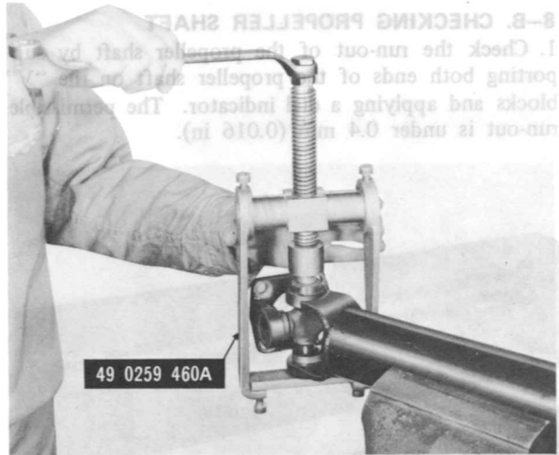
Fig. 8-7 Installing universal joint
