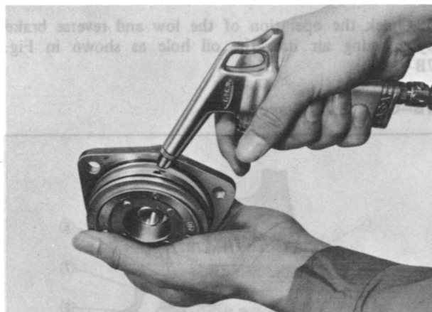
Fig. 7B-34 Blowing out piston
