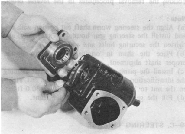
Fig. 10-9 Installing end cover and adjusting shim
