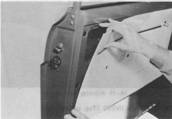
Fig. 14-6 Removing trim board
