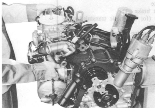
Fig. 1-95 Installing intake manifold assembly
