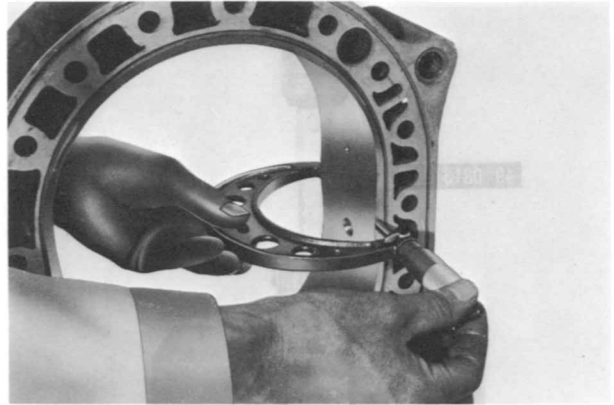
Fig. 1-39 Checking rotor housing width
