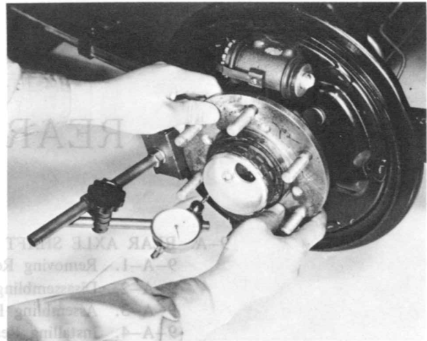
Fig. 9-1 Checking end play
