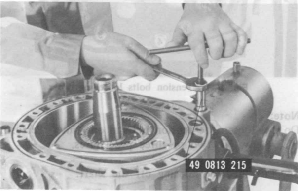
Fig. 1-20 Removing tubular dowel
