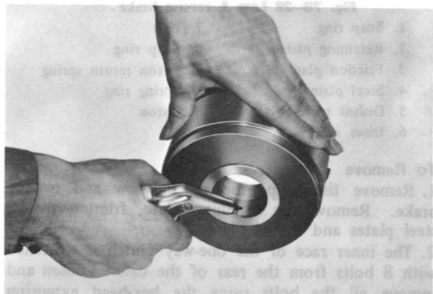
Fig. 7B-21 Blowing out piston
