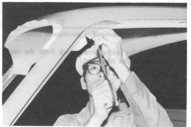
Fig. 14-17 Trimming headlining material
