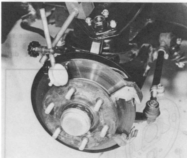
Fig. 11-43 Checking rotor run-out
