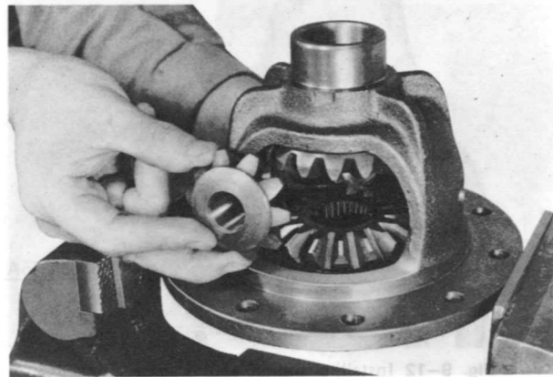
Fig. 9-18 Installing differential gears
