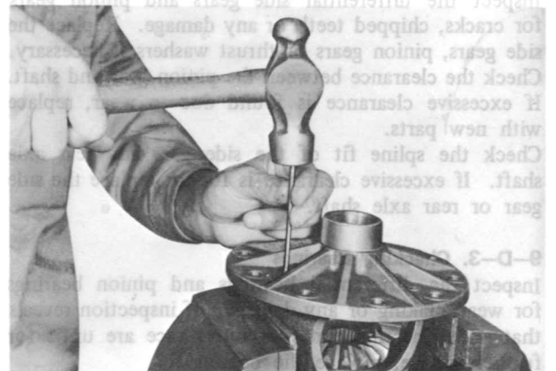
Fig. 9-7 Removing pinion shaft lock pin
