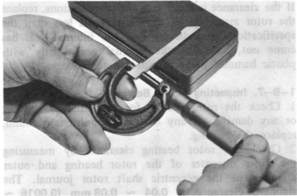
Fig. 1-47 Checking apex seal
