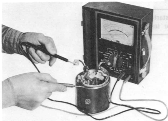
Fig. 5-41 Checking field coil for ground
