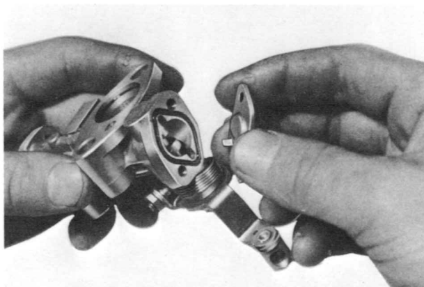
Fig. 2-28 Fitting rear plate
