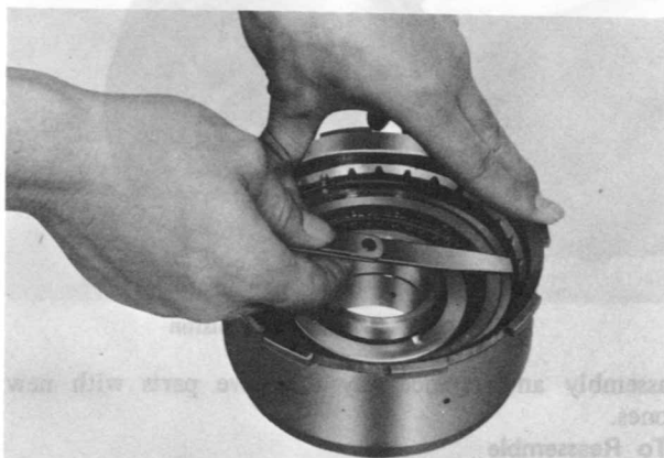
Fig. 7B-22 Measuring clearance
