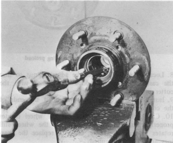
Fig. 12-9 Removing inner bearing cup
