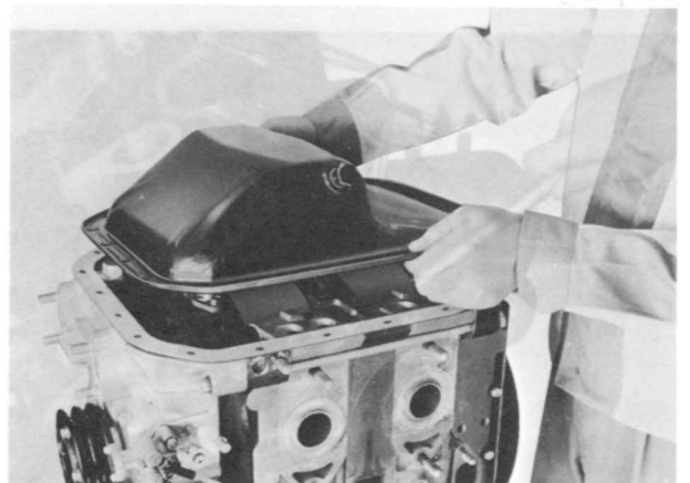
Fig. 1-8 Removing oil pan
