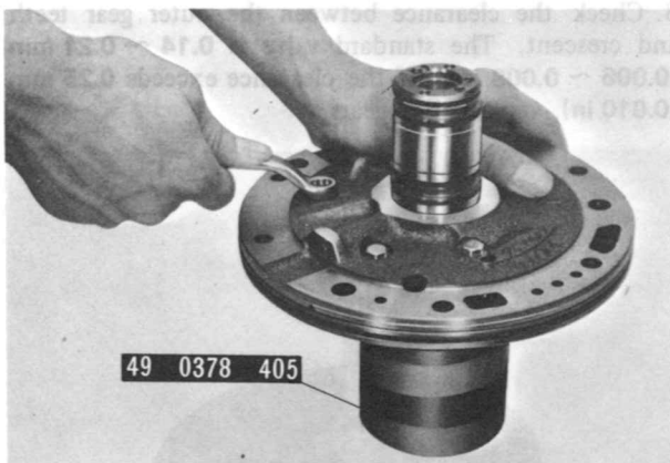
Fig. 7B-43 Assembling oil pump
