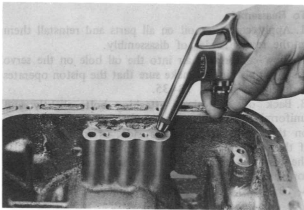
Fig. 7B-29 Blowing out piston
