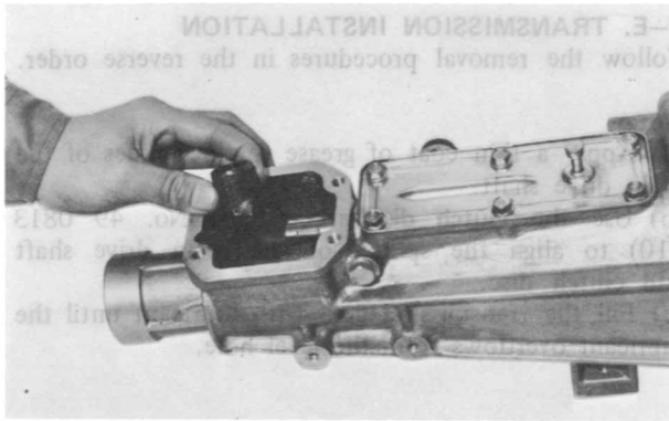
Fig. 7-35 Installing control lever end
