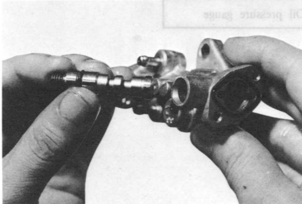
Fig. 2-27 Inserting control pin
