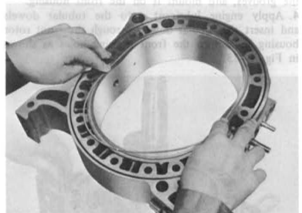
Fig. 1-70 Installing sealing rubber
