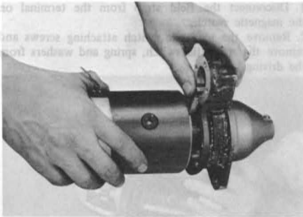
Fig. 5-35 Removing yoke assembly
