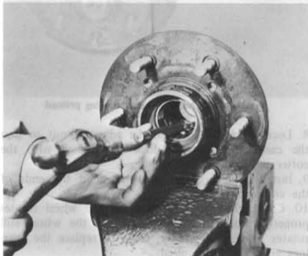
Fig. 12-9 Removing inner bearing cup
