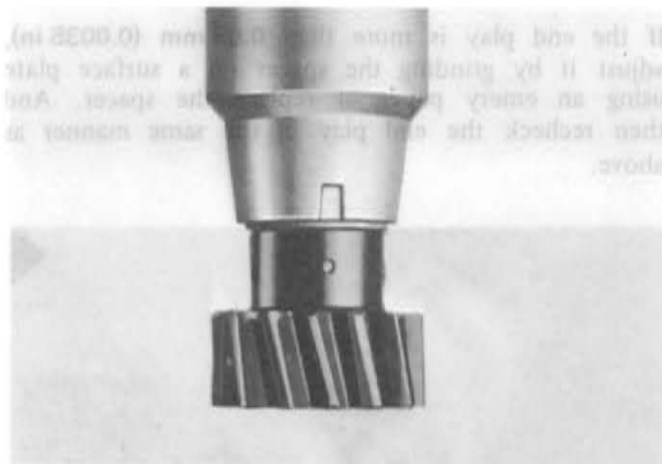
Fig. 1-93 Aligning tally mark
