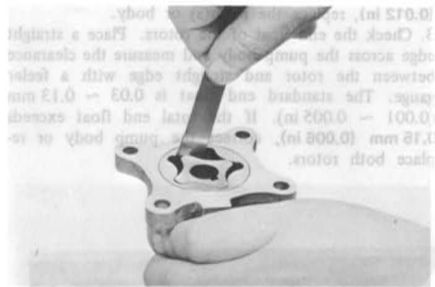
Fig. 2-3 Checking rotor clearance
