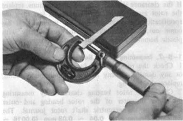
Fig. 1-47 Checking apex seal
