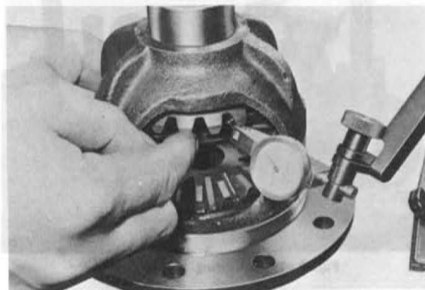
Fig. 9-19 Checking backlash of pinion and side gear
