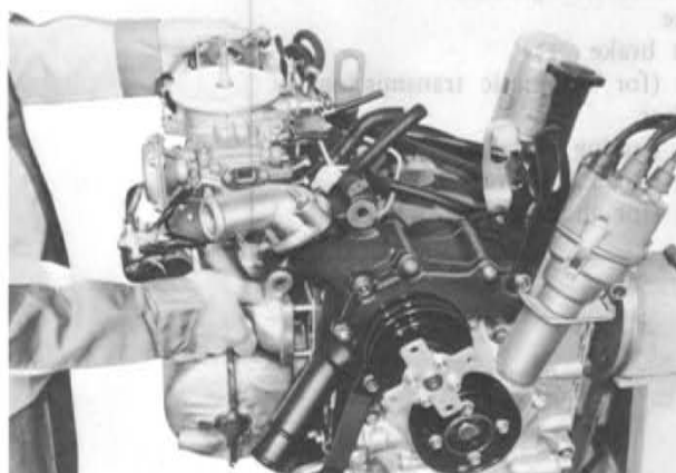
Fig. 1-95 Installing intake manifold assembly
