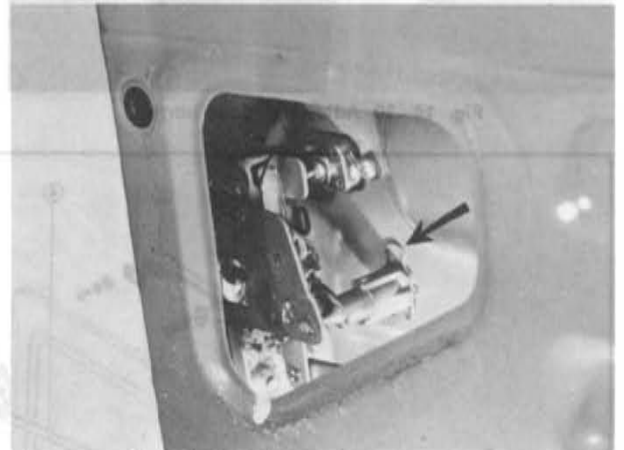
Fig. 14-9 Prying cylinder retainer
