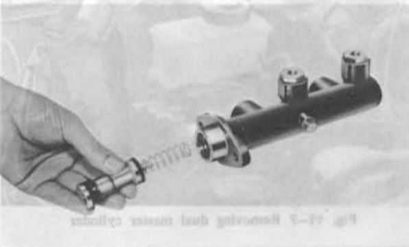
Fig. 11-10 Removing primary piston
