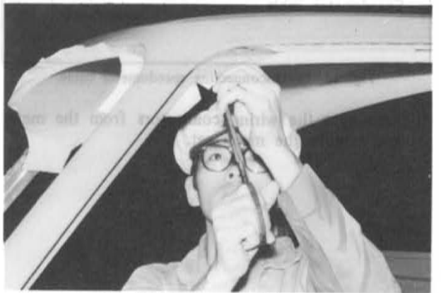
Fig. 14-17 Trimming headlining material
