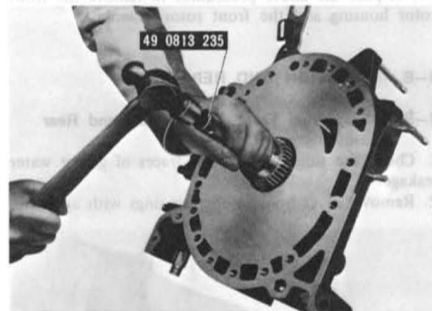
Fig. 1-31 Removing stationary gear assembly
