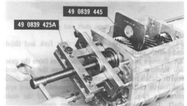
Fig. 7-5 Removing counter shaft front bearing
