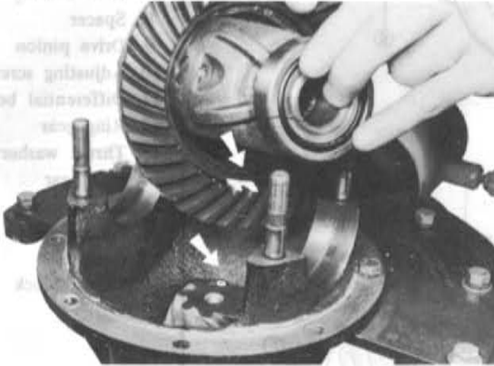
Fig. 9-23 Installing of differential assembly
