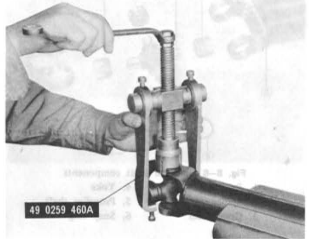
Fig. 8-4 Removing universal joint
