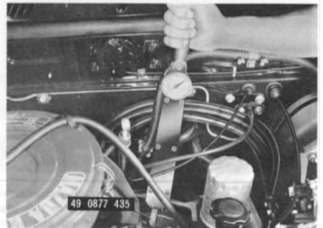
Fig. 7B-59 Tightening torque converter
