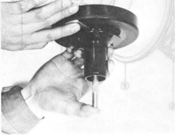
Fig. 11-24 Removing retainer key
