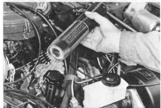
Fig. 1A-48 Checking control unit (I)
