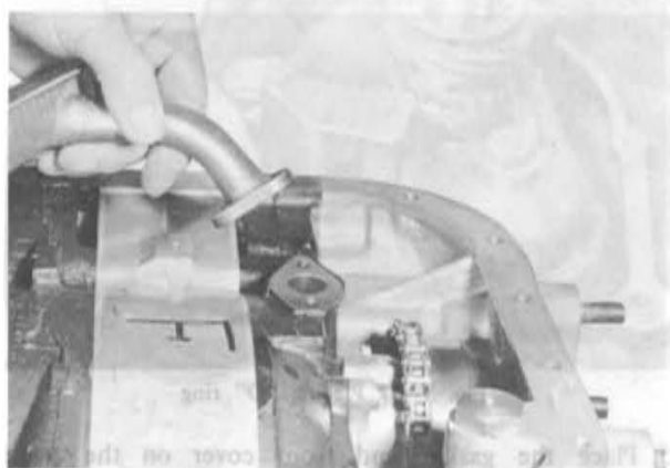
Fig. 1-90 Installing oil strainer
