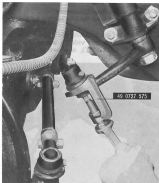
Fig. 10-4 Disconnecting center link
