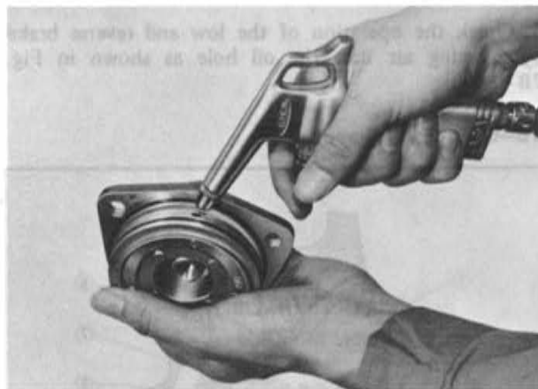
Fig. 7B-34 Blowing out piston
