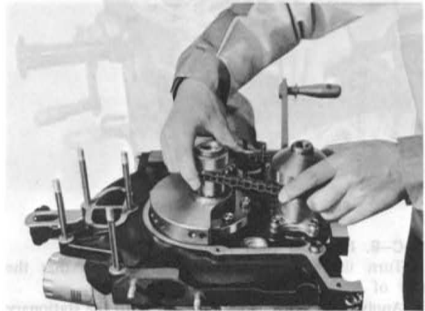
Fig. 1-83 Installing chain and sprockets
