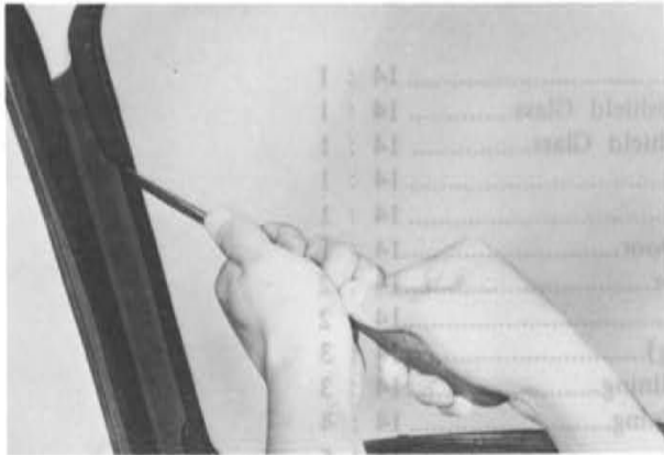
Fig. 14-1 Pushing out inner lip of weatherstrip
