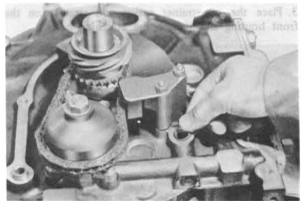
Fig. 1-87 Placing "O" ring
