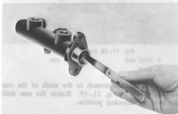
Fig. 11-14 Checking piston clearance
