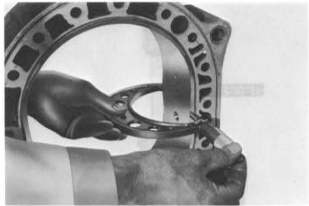
Fig. 1-39 Checking rotor housing width
