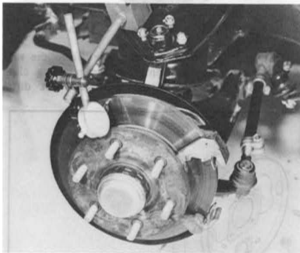
Fig. 11-43 Checking rotor run-out
