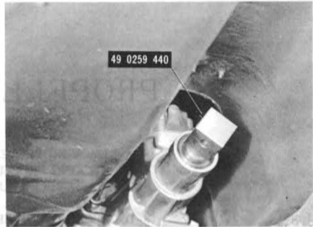
Fig. 8-1 Holder installed into extension housing
