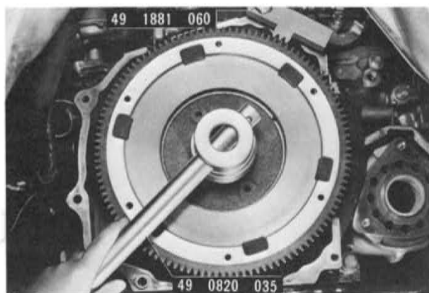
Fig. 6-2 Loosening flywheel nut
