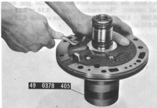
Fig. 7B-43 Assembling oil pump
