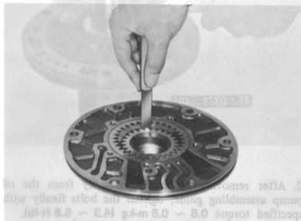
Fig. 7B-41 Measuring clearance (2)
