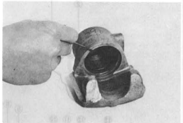
Fig. 11-39 Removing piston seal
