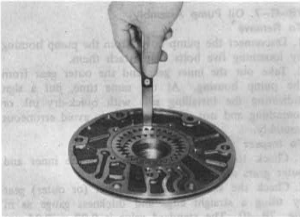
Fig. 7B-42 Measuring clearance (3)
