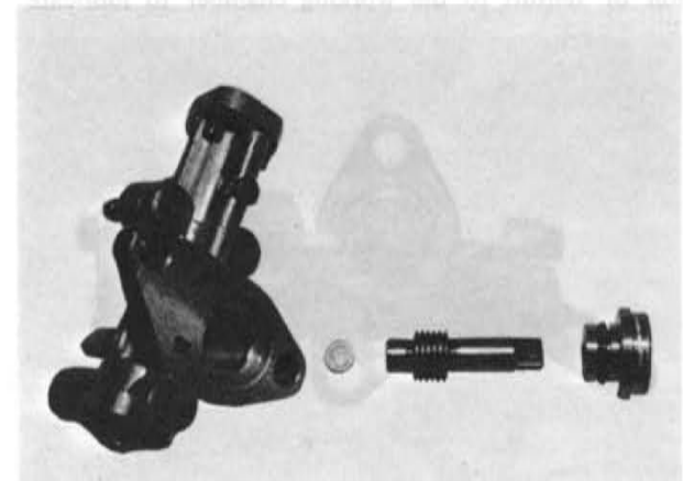
Fig. 2-25 Assembling drive worm
