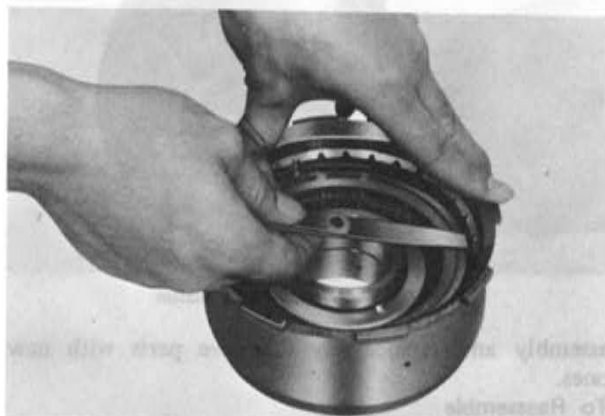
Fig. 7B-22 Measuring clearance
