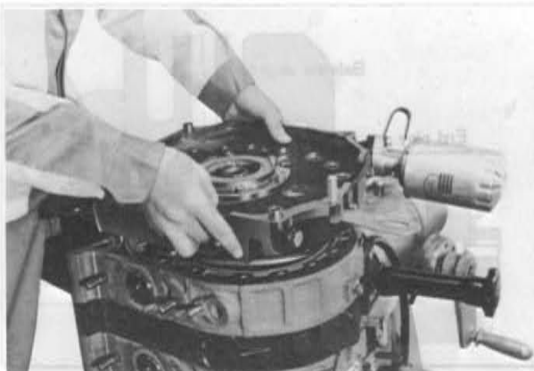
Fig. 1-78 Installing rear housing
