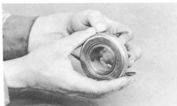
Fig. 6-4 Checking release bearing
