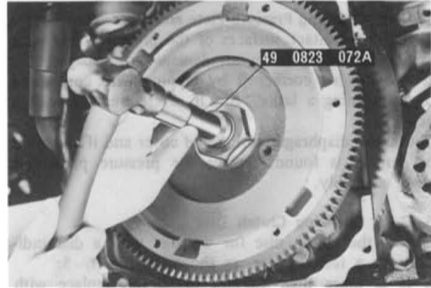
Fig. 6-10 Installing pilot bearing
