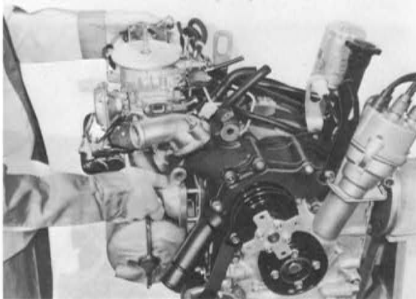
Fig. 1-5 Removing intake manifold ass'y
