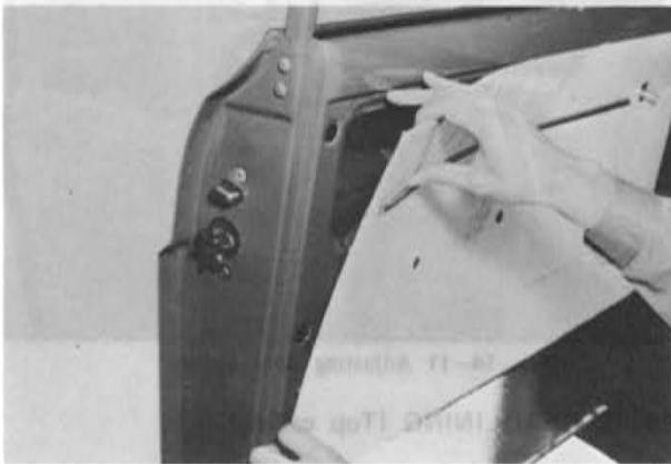
Fig. 14-6 Removing trim board
