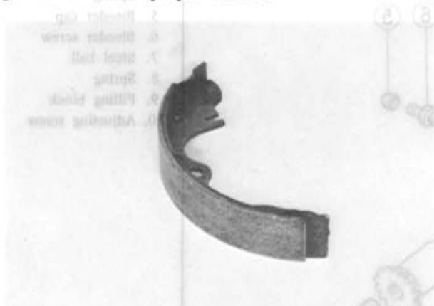
Fig. 11-52 Rear brake shoe
