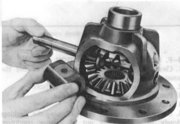
Fig. 9-20 Installing thrust block and pinion shaft
