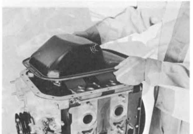
Fig. 1-8 Removing oil pan
