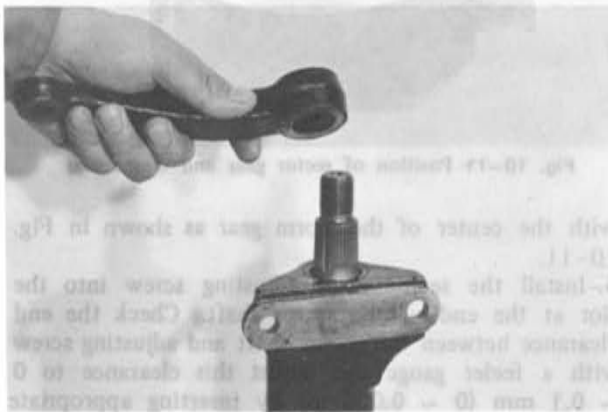
Fig. 10-14 Installing pitman arm
