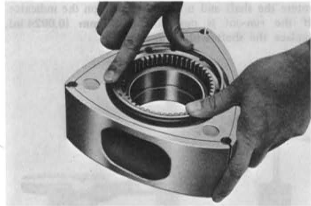
Fig. 1-64 Installing oil seal
