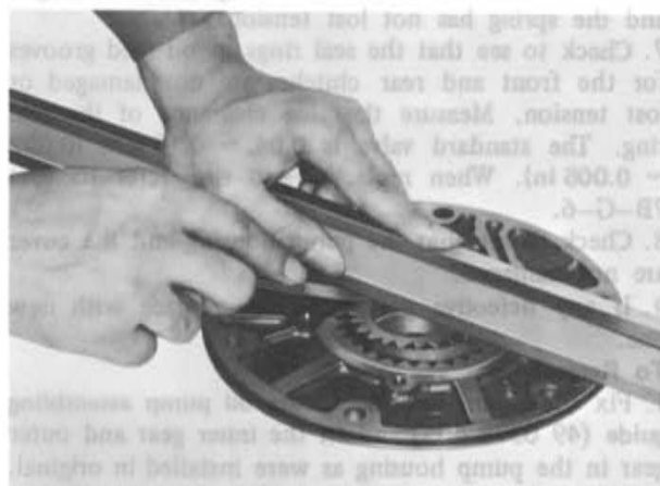
Fig. 7B-40 Measuring clearance (1)
