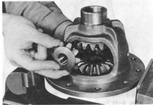
Fig. 9-18 Installing differential gears
