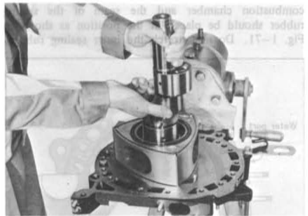
Fig. 1-68 Installing eccentric shaft
