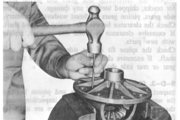
Fig. 9-7 Removing pinion shaft lock pin
