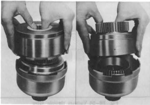
Fig. 7B-49 Assembling clutches
