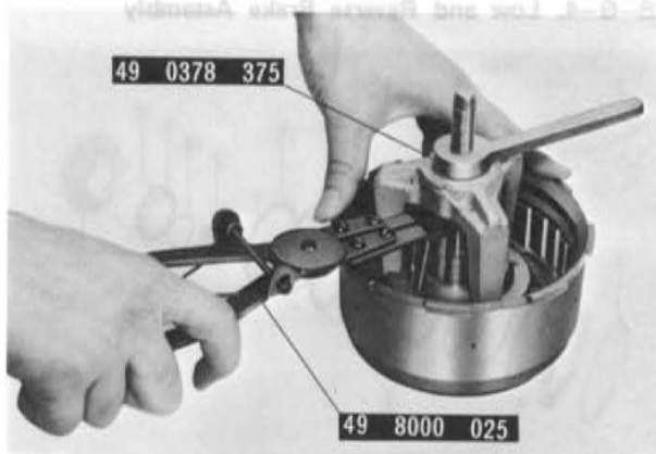
Fig. 7B-20 Removing snap ring
