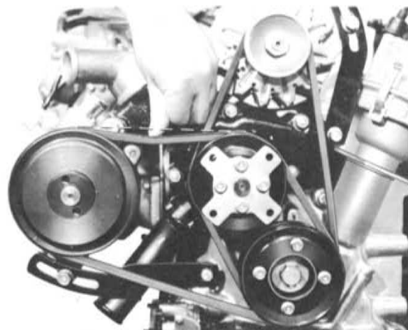
Fig. 1-98 Adjusting air pump belt
