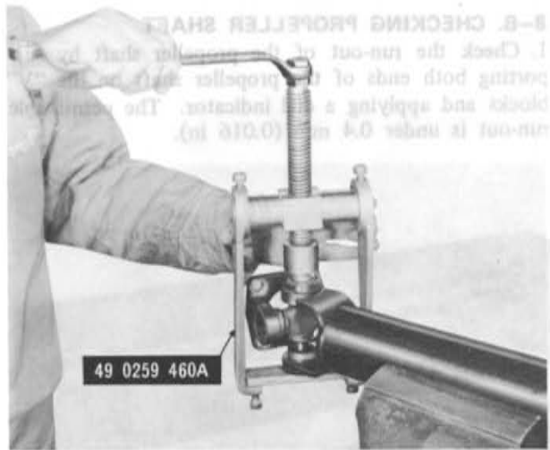
Fig. 8-7 Installing universal joint
