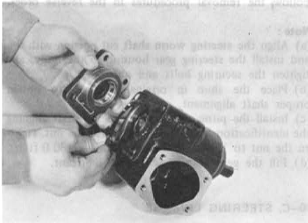
Fig. 10-9 Installing end cover and adjusting shim
