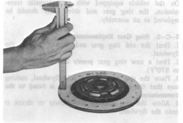
Fig. 6-6 Checking clutch disc for wear
