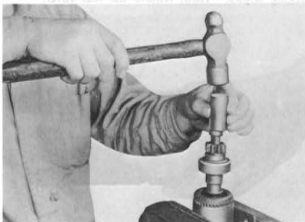
Fig. 5-37 Removing pinion stop collar
