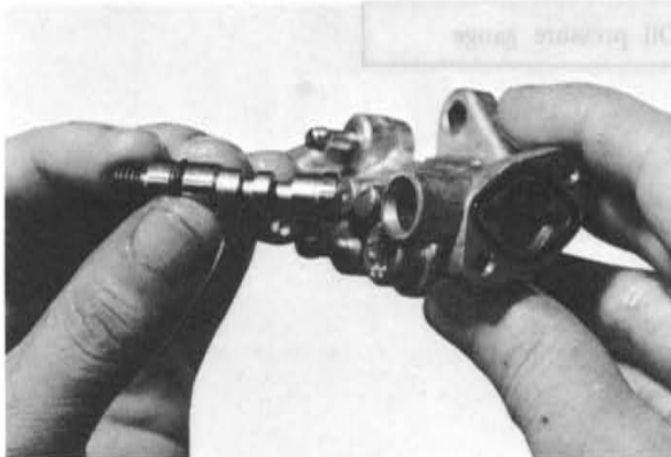
Fig. 2-27 Inserting control pin
