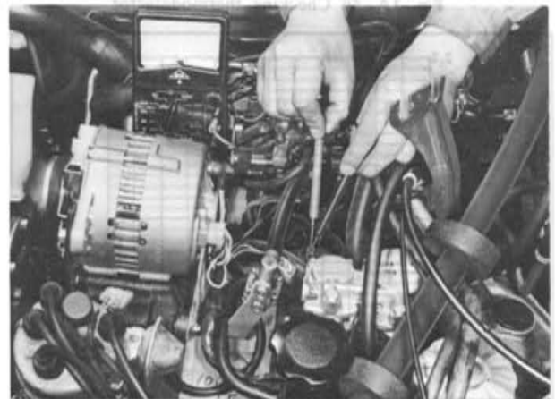
Fig. 1A-43 Checking thermosensor
