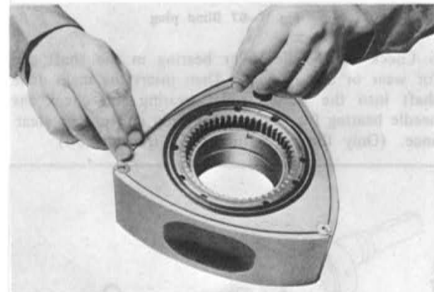
Fig. 1-65 Installing side seal
