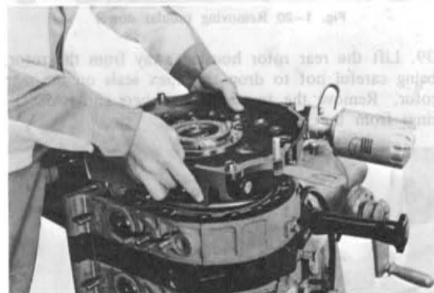
Fig. 1-18 Removing rear housing
