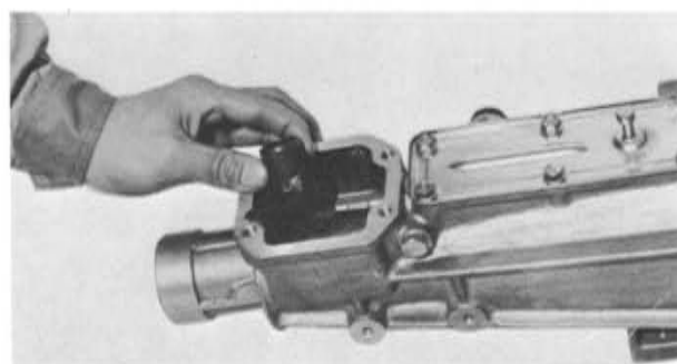
Fig. 7-2 Removing control lever end
