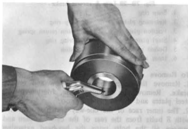
Fig. 7B-21 Blowing out piston
