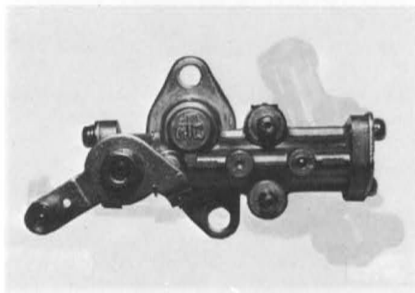
Fig. 2-20 Metering oil pump
