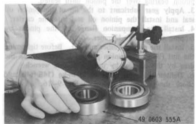
Fig. 9-14 Measuring bearing height
