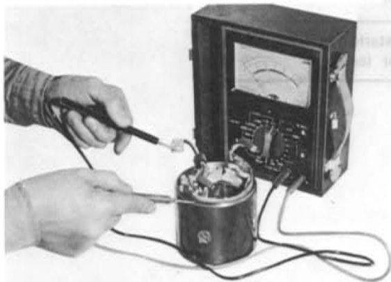
Fig. 5-41 Checking field coil for ground
