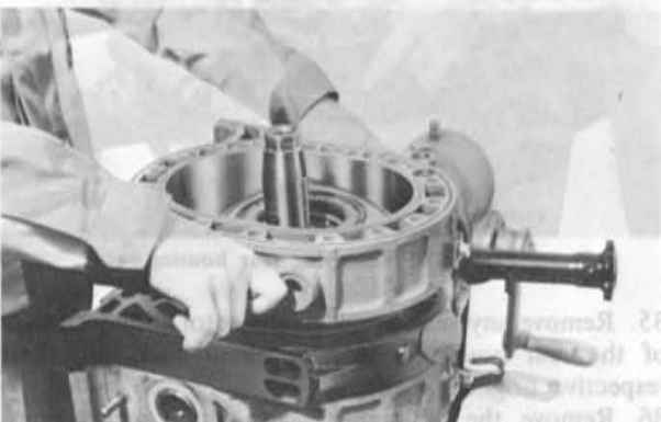
Fig. 1-21 Removing rear rotor housing
