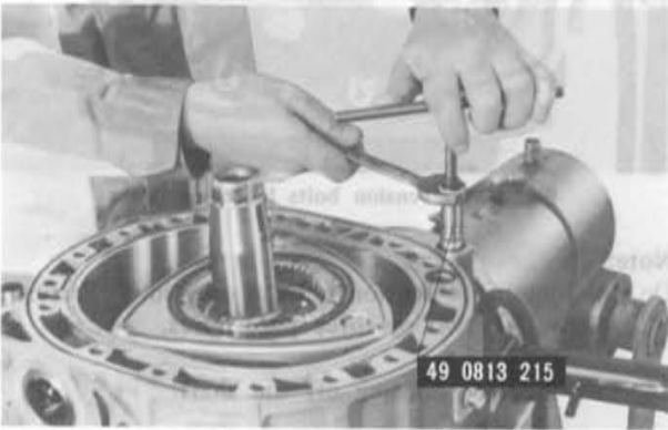
Fig. 1-20 Removing tubular dowel
