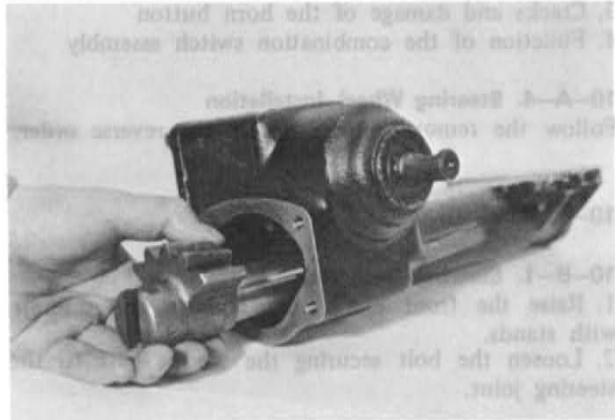
Fig. 10-6 Removing sector shaft
