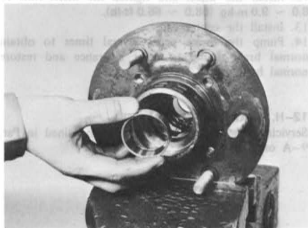
Fig. 12-10 Installing outer bearing cup
