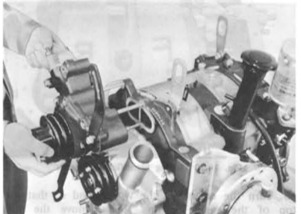
Fig. 1-7 Removing water pump
