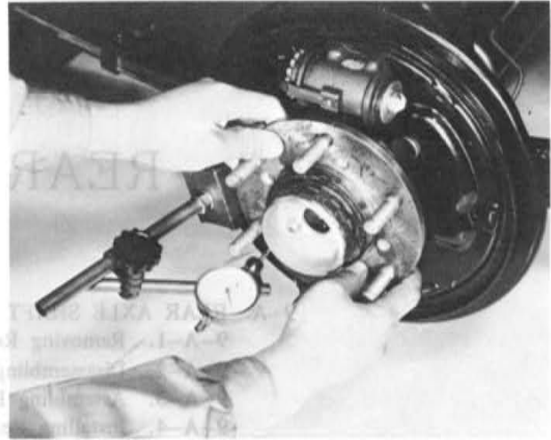
Fig. 9-1 Checking end play
