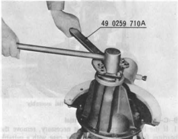
Fig. 9-8 Loosening pinion nut
