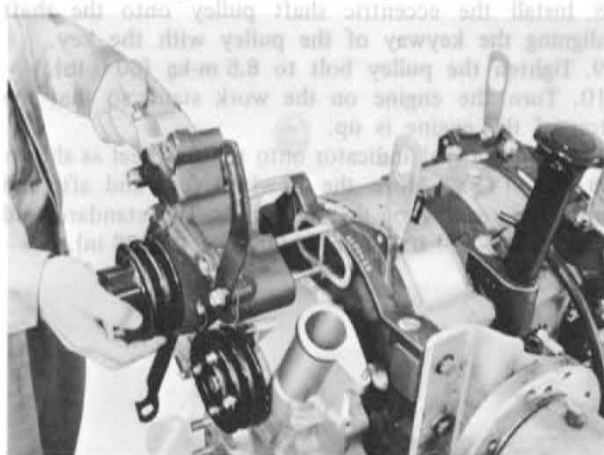
Fig. 1-92 Installing water pump
