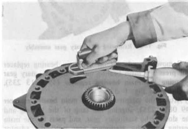
Fig. 1-26 Removing sealing agent
