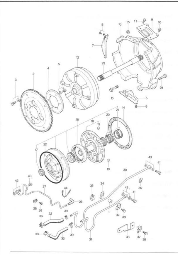
(CONVERTER, OIL PUMP & PIPING)
