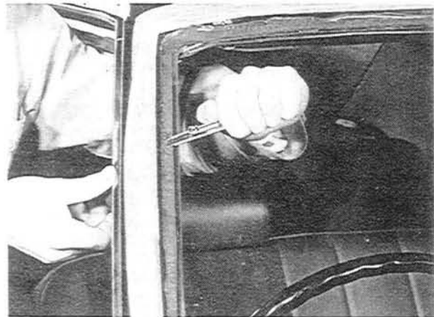
Fig. 14-7 Cutting of sealant
