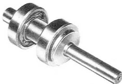
Fig. 3-4 Bearing and shaft assembly
