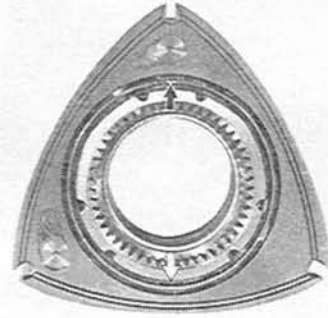
Fig. 1-74 Position of spring gap
