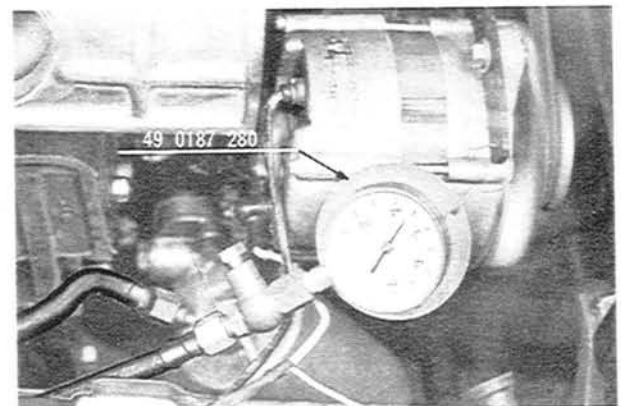
Fig. 2-3 Checking of oil pressure.
