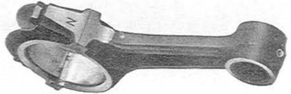
Fig. 1-33 Mark of connecting rod weight
