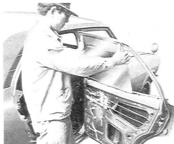
Fig. 14-26 Removing of glass
