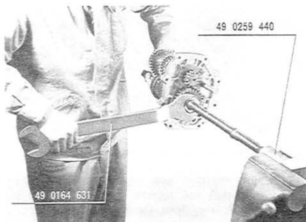
Fig. 7-11 Loosening of lock nut
