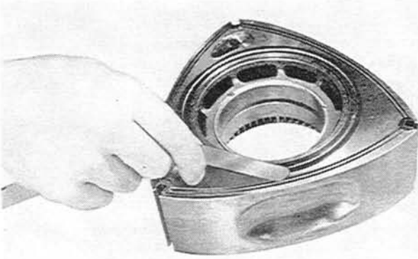
Fig. 1-63 Checking side seal gap
