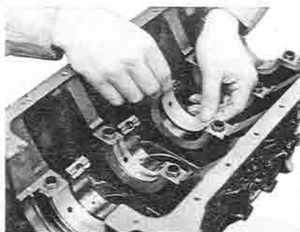
Fig. 1-47 Installing of main bearing
