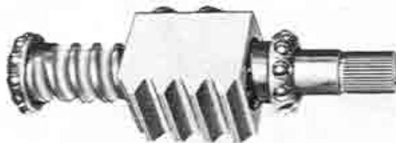
Fig. 10-5 Worm and ball nut assembly
