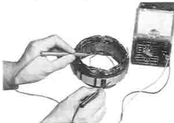
Fig. 5-10 Checking of stator coil for ground
