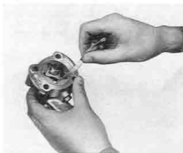
Fig. 2-4 Checking gap of rotors
