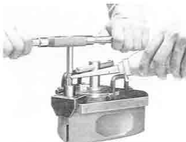
Fig. 1-67 Reboring corner seal groove
