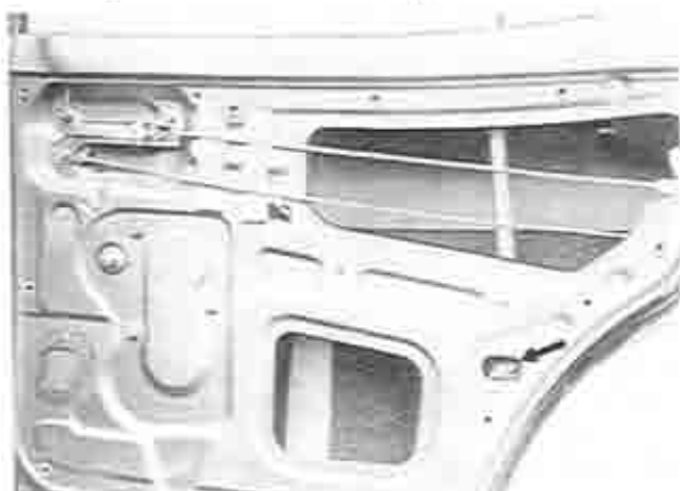
Fig. 14-25 Removing of center sash
