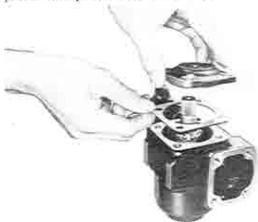
Fig. 10-6 Installing of end cover and shim.
