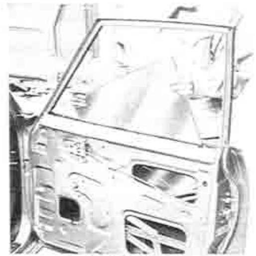
Fig. 14-20 Removing of glass
