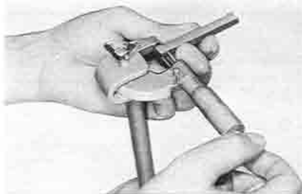
Fig. 1-60 Measuring apex seal height
