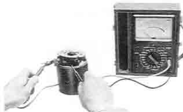
Fig. 5-28 Checking of field coil for ground
