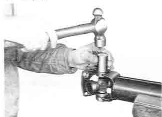
Fig. 8-3 Removing of bearing cup
