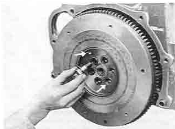
Fig. 6-6 Installing of flywheel
