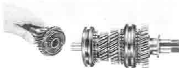
Fig. 7-21 Installing of main drive shaft
