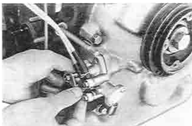
Fig. 1-98 Installing metering pump
