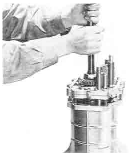
Fig. 7-25 Installing of bearing housing
