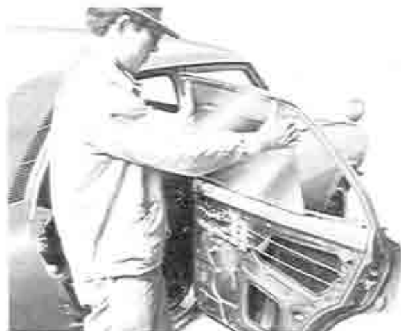
Fig. 14-26 Removing of glass
