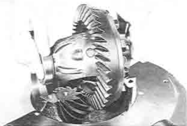
Fig. 9-10 Removing of differential assembly
