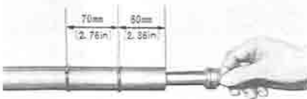
Fig. 13-19 Installing of oil stop rings
