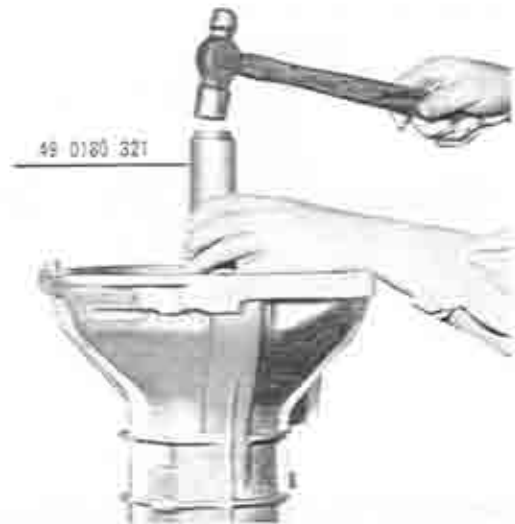
Fig. 7A-20 Installing of bearings
