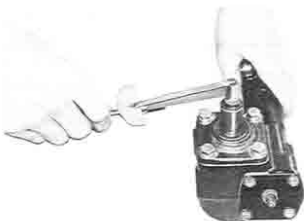
Fig. 10-11 Checking of preload
