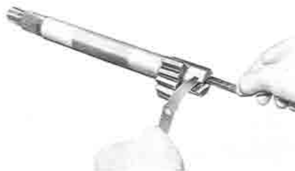
Fig. 10-7 Checking of end clearance
