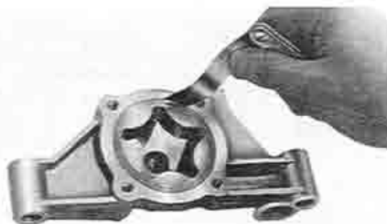
Fig. 2-5 Checking of rotor and body clearance
