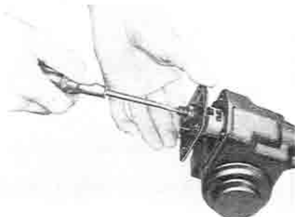
Fig. 10-9 Installing of side cover
