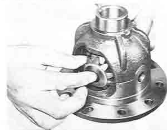
Fig. 9-23 Installing of pinion gears
