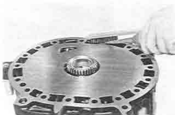
Fig. 1-28 Cleaning front housing
