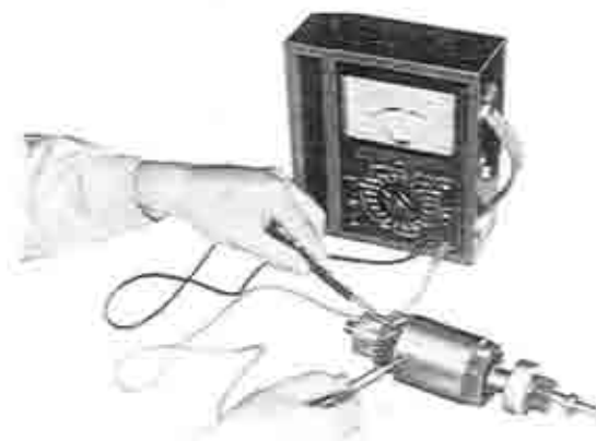
Fig. 5-26 Checking of armature
