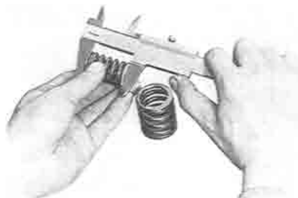
Fig. 1-12 Checking of free length
