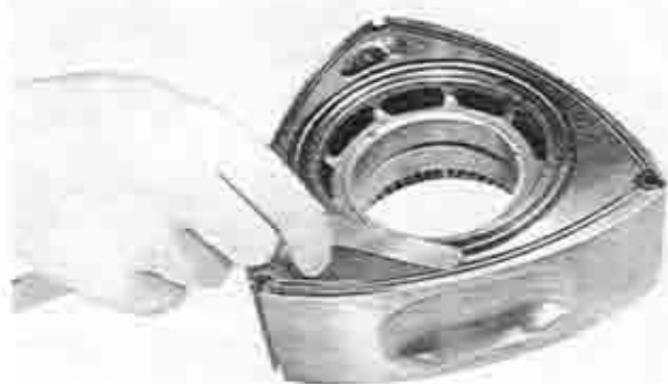
Fig. 1-63 Checking side seal gap
