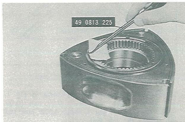
Fig. 1-67 Removing of oil seal
