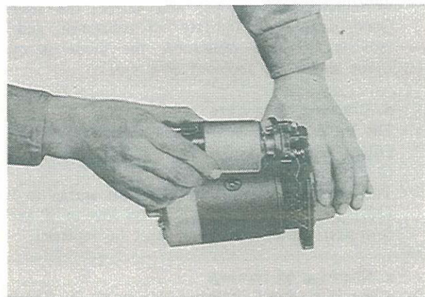
Fig. 5-19 Removing of magnetic switch
