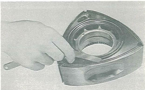
Fig. 1-73 Checking of side seal gap
