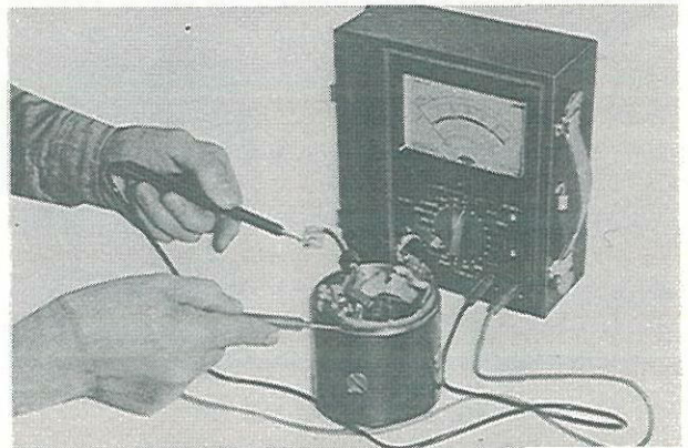
Fig. 5-22 Checking of field coil
