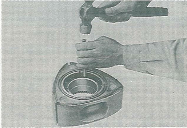
Fig. 1-62 Staking of locking screws
