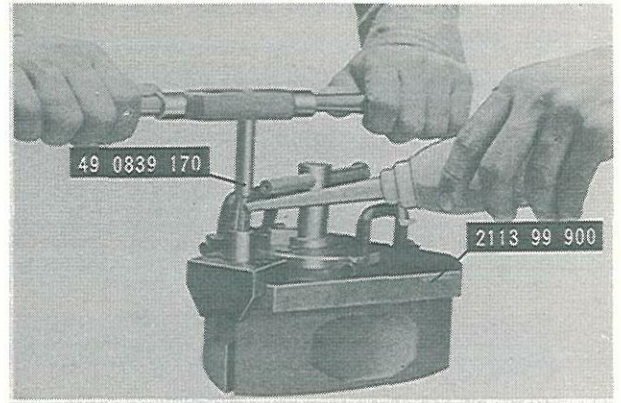
Fig. 1-77 Reaming of corner seal groove
