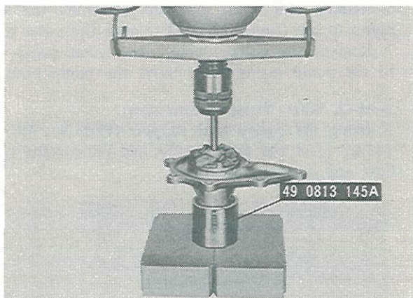
Fig. 3-12 Removing of impeller
