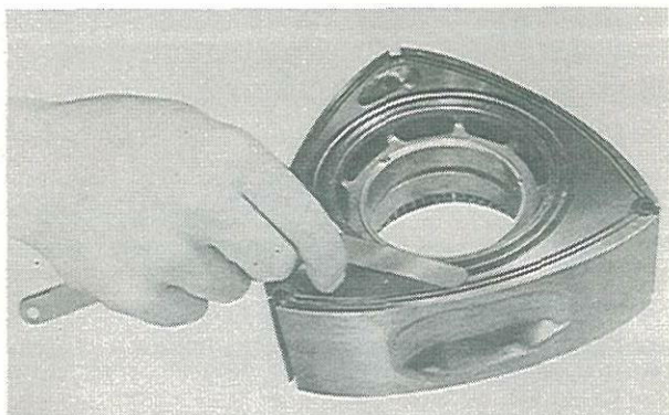
Fig. 1-73 Checking of side seal gap
