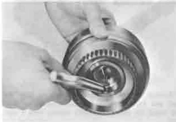
Fig. 7B-30 Blowing out piston
