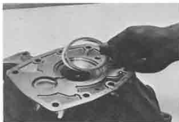
Fig. 7A-76 Installing shim
