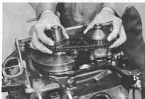
Fig. 1-80 Installing oil pump drive chain and sprockets
