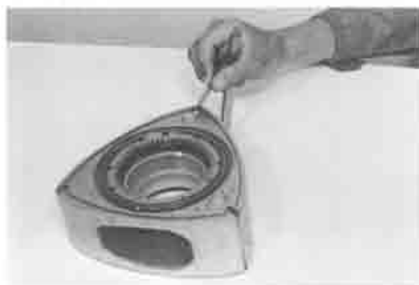
Fig. 1-48 Checking seal clearance
