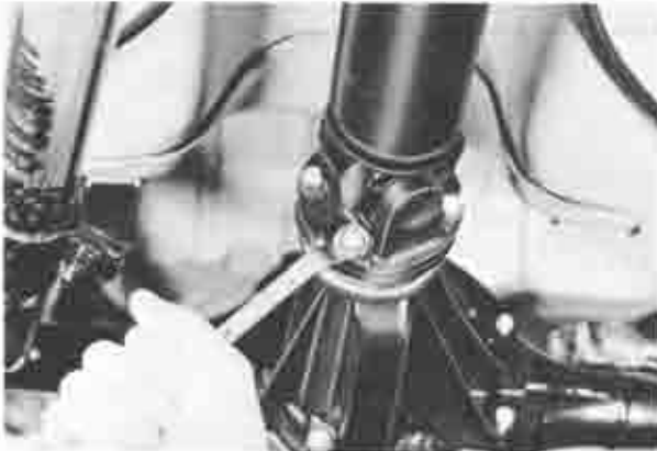
Fig. 8-1 Removing propeller shaft attaching bolts
