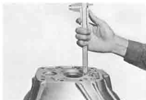
Fig. 7-35 Measuring bearing bore depth
