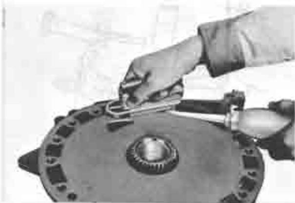
Fig. 1-24 Cleaning front housing
