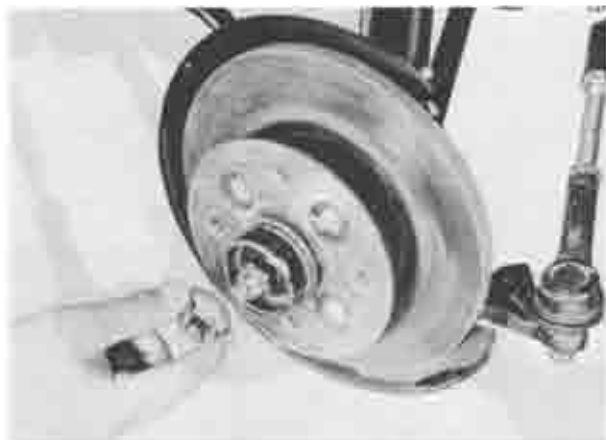
Fig. 12-6 Installing nut lock
