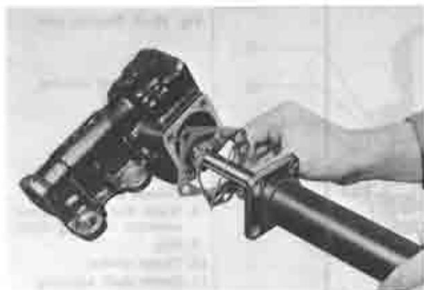
Fig. 10-8 Installing column jacket and shims
