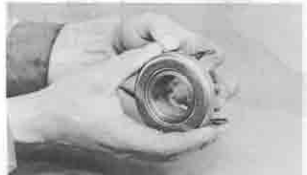
Fig. 6-5 Checking release bearing
