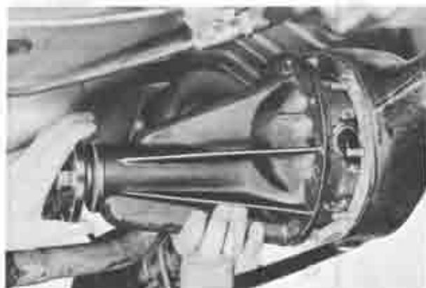
Fig. 9-10 Removing rear axle assembly
