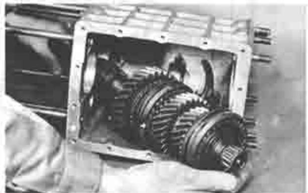
Fig. 7A-49 Installing main shaft and gear assembly
