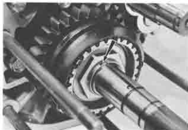
Fig. 7A-26 Main shaft lock nut tab
