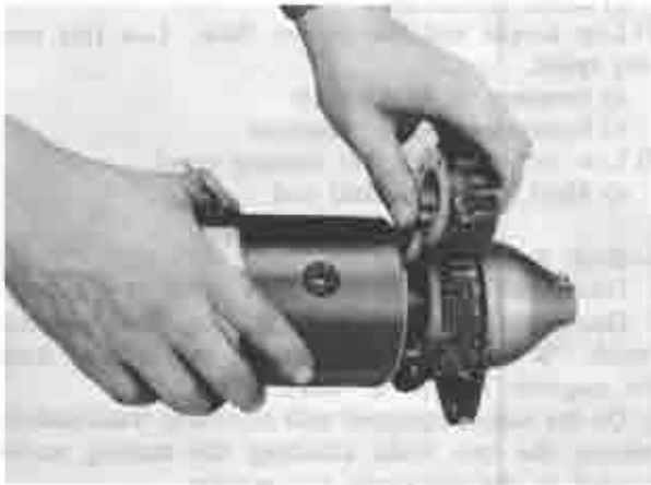
Fig. 5-21 Removing yoke assembly
