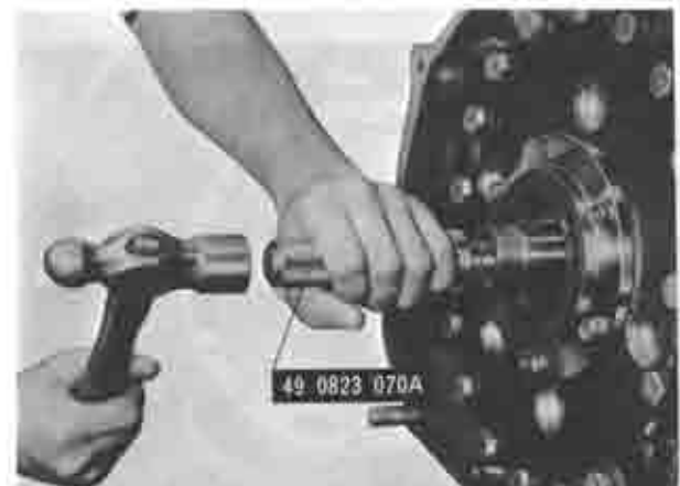
Fig. 6-9 Installing roller bearing
