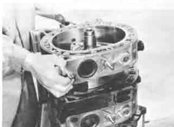
Fig. 1-70 Installing rear rotor housing
