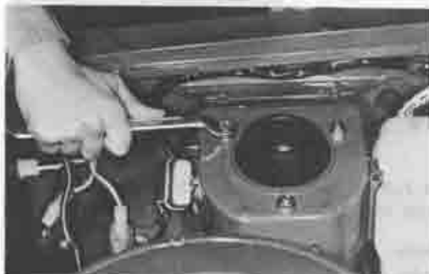
Fig. 13-3 Removing attaching nuts
