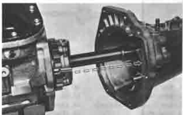
Fig. 7B-59 Installing extension housing
