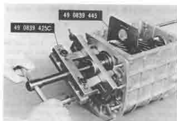
Fig. 7A-29 Removing counter shaft front bearing
