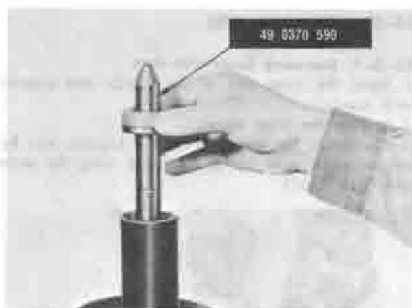
Fig. 13-10 Installing cap nut
