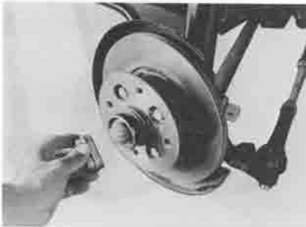
Fig. 12-2 Removing grease cap
