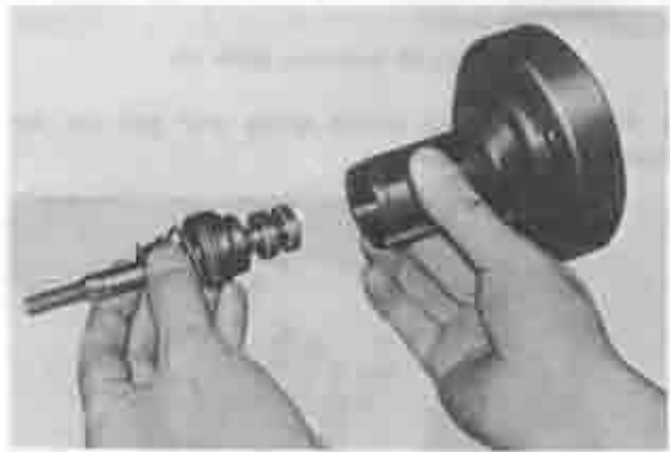
Fig. 11-19 Removing valve rod assembly
