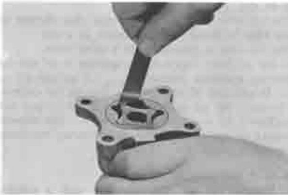
Fig. 2-9 Checking rotor clearance
