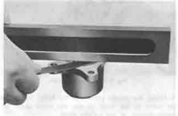
Fig. 2-11 Checking end float
