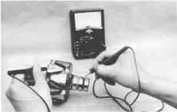
Fig. 5-9 Checking rotor for ground
