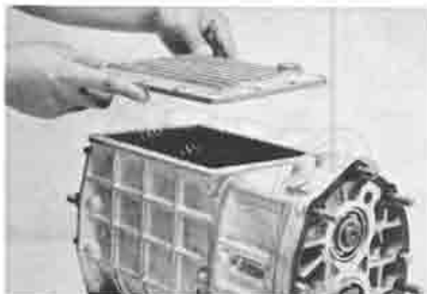
Fig. 7A-10 Removing under cover
