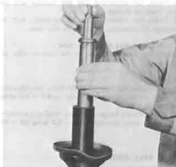
Fig. 13-9 Installing tube and rod assembly
