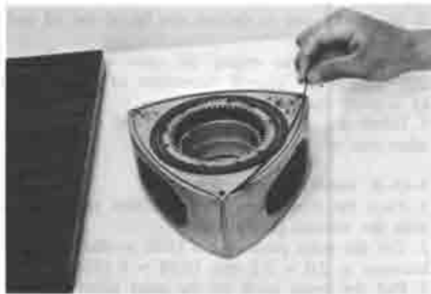
Fig. 1-56 Installing side seal
