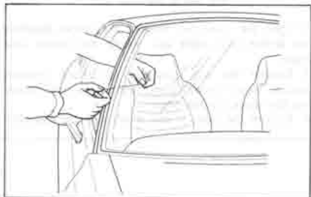
Fig. 14-20 Piercing piano wire
