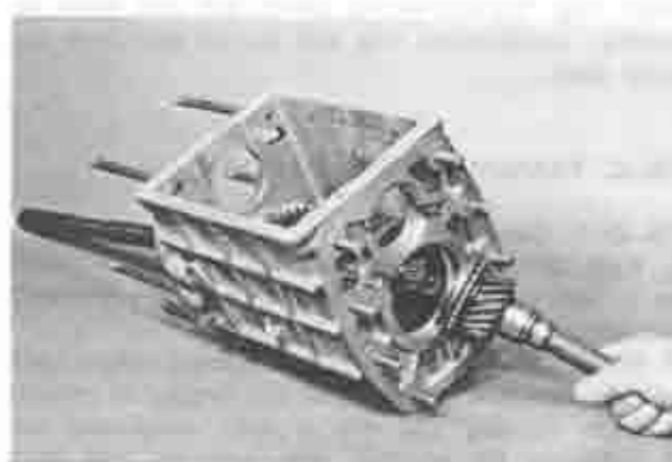
Fig. 7A-34 Removing main drive shaft
