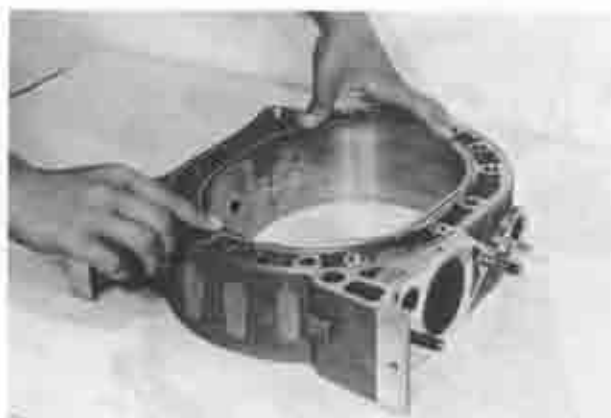
Fig. 1-62 Installing sealing rubber
