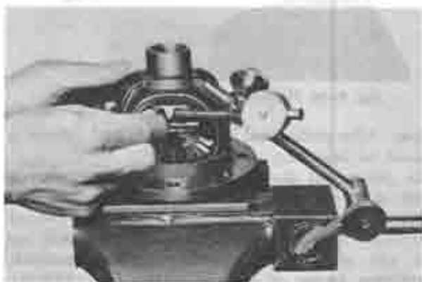
Fig. 9-26 Checking backlash of pinion and side gear
