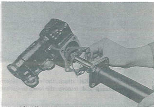
Fig. 10-8 Installing of column jacket and shims
