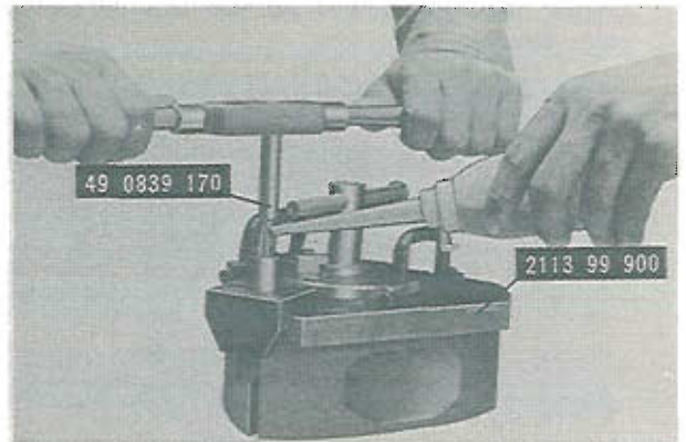
Fig. 1-77 Reaming of corner seal groove
