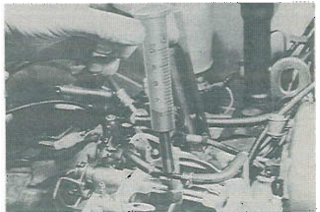
Fig. 2-12 Checking of oil discharge
