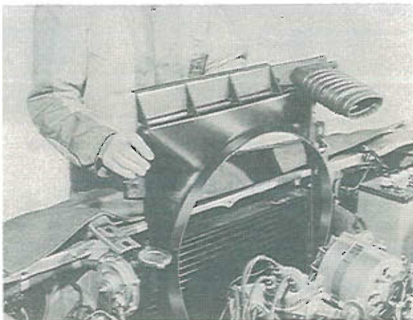
Fig. 3-3 Removing of radiator shroud
