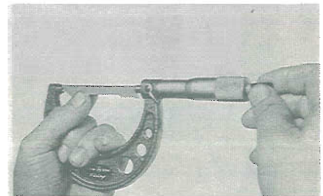
Fig. 1-49 Measuring apex seal length
