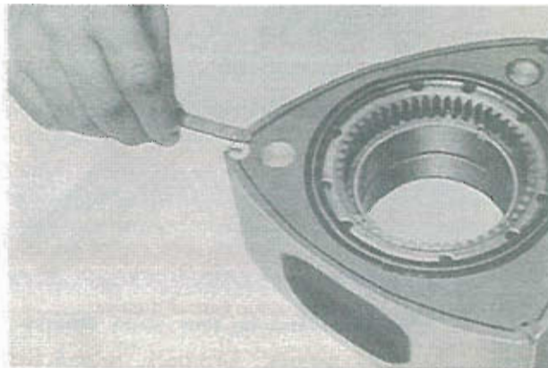
Fig. 1-52 Checking corner seal and side seal gap
