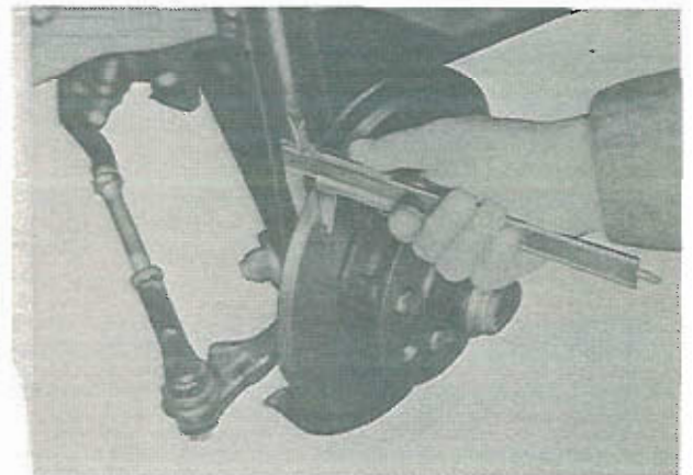
Fig. 11-46 Checking of rotor thickness
