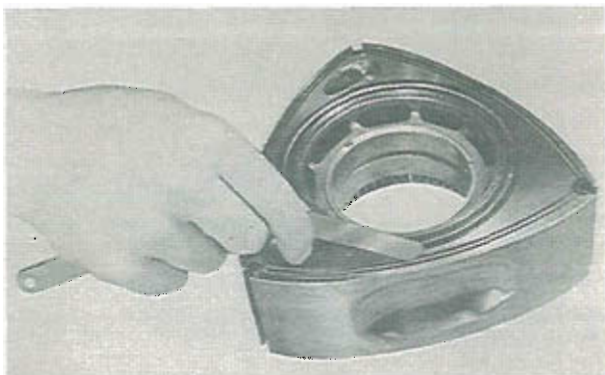
Fig. 1-73 Checking of side seal gap
