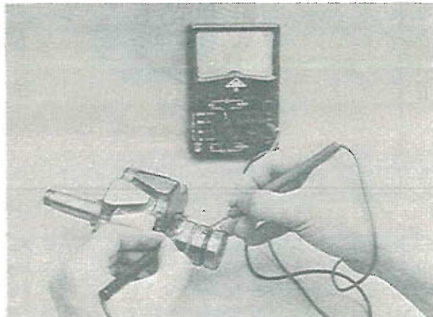
Fig. 5-22 Checking rotor for open
