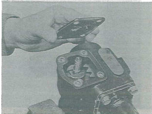
Fig. 10-12 Placing of side cover
