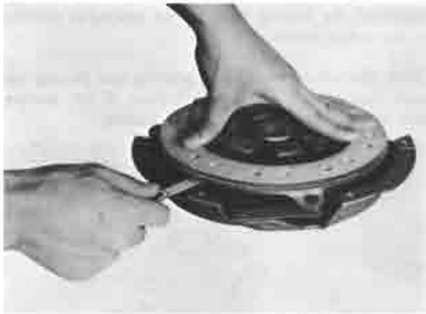
Fig. 6-9 Checking clutch disc for warpage
