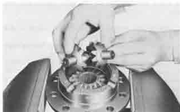
Fig. 9-29 Installing differential gears
