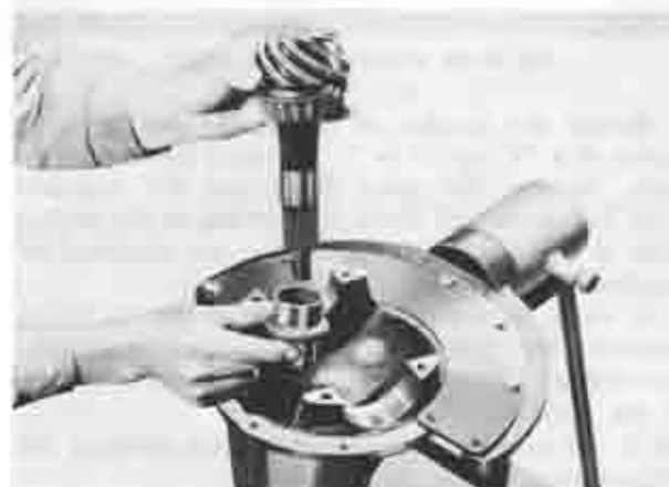
Fig. 9-26 Installing pinion and collapsible spacer
