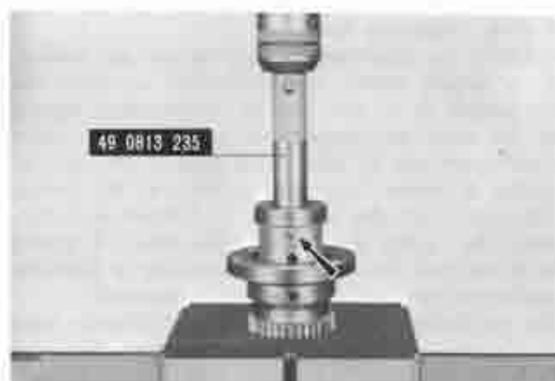
Fig. 1-33 Installing main bearing
