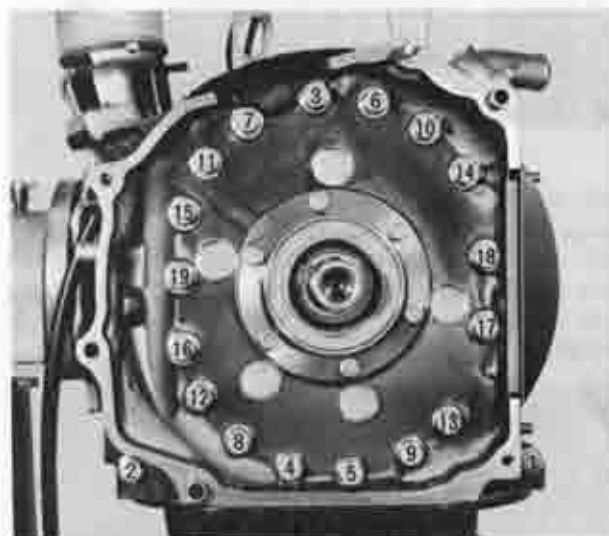
Fig. 1-17 Tension bolts loosening order
