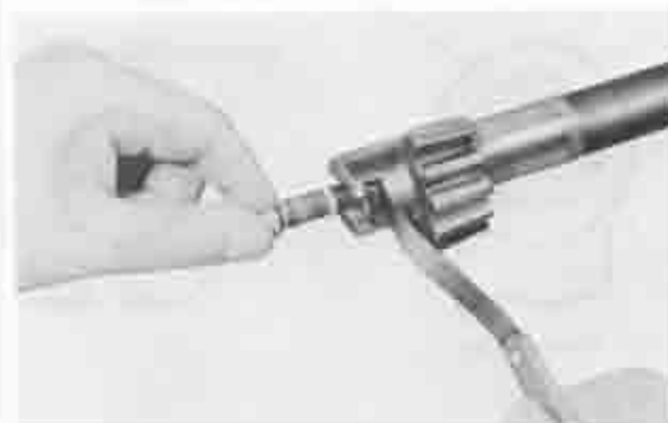
Fig. 10-13 Checking end clearance
