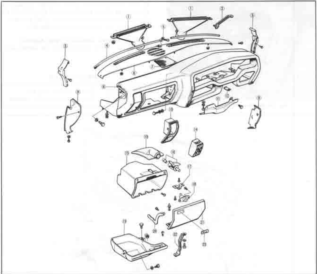
Fig. 14-109 Instrument panel components (Right hand drive vehicles)
