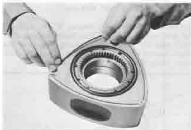
Fig. 1-65 Installing side seal
