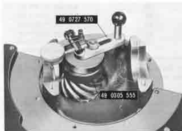
Fig. 9-24 Measuring pinion height
