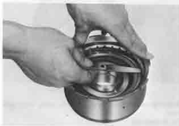
Fig. 7B-22 Measuring clearance
