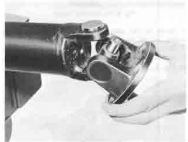
Fig. 8-22 Installing yoke and spider assembly
