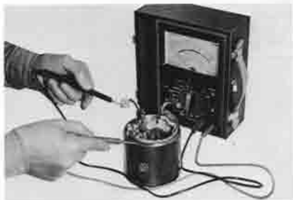
Fig. 5-41 Checking field coil for ground
