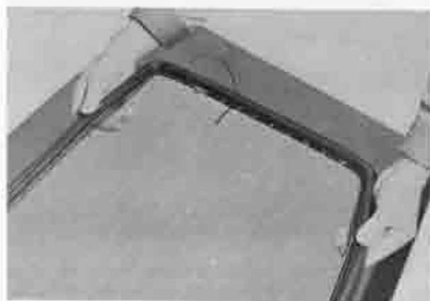
Fig. 14A-19 Installing weatherstrip
