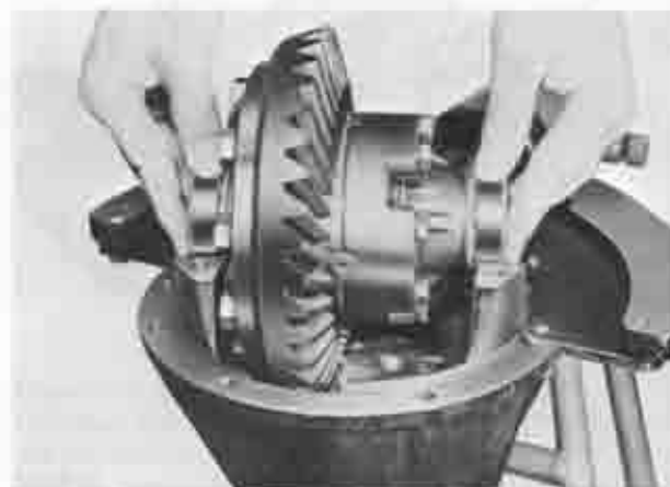
Fig. 9-32 Installing differential assembly
