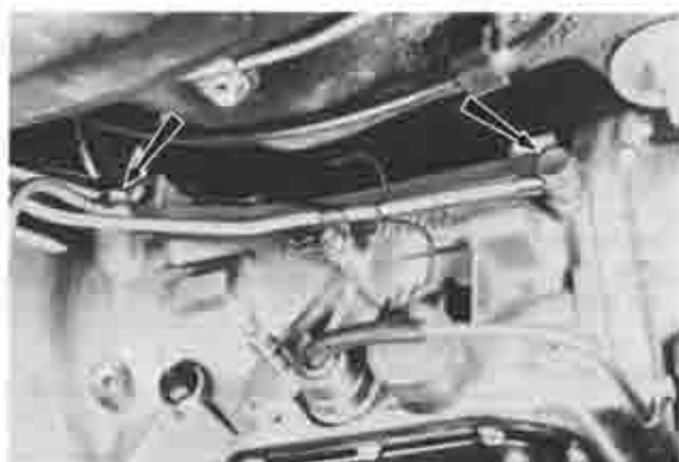
Fig. 7B-10 Removing pipes
