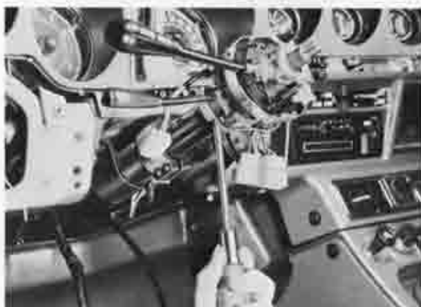
Fig. 15-25 Removing combination switch
