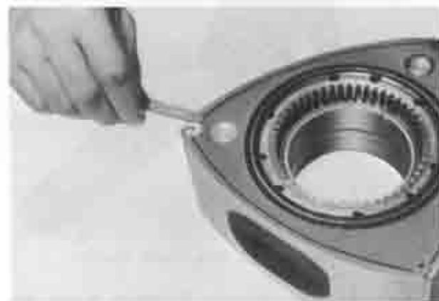
Fig. 1-52 Checking corner seal and side seal gap
