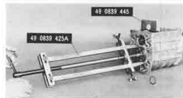
Fig. 7C-27 Removing main drive shaft bearing
