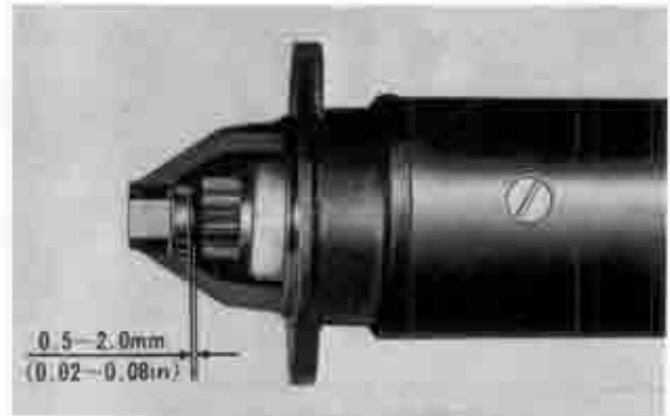
Fig. 5-45 Checking pinion position
