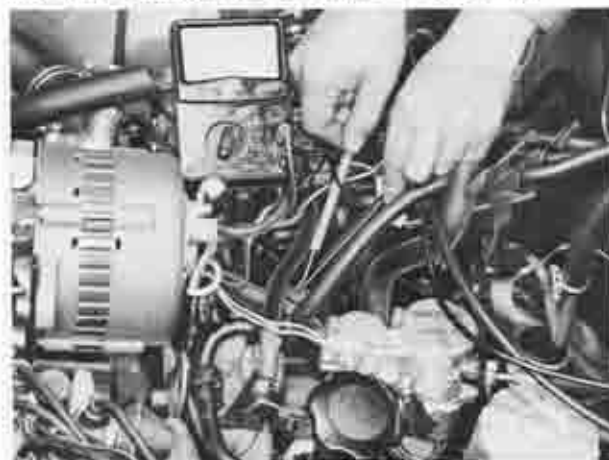
Fig. 1A-44 Checking thermosensor
