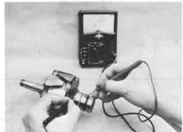
Fig. 5-22 Checking rotor for open
