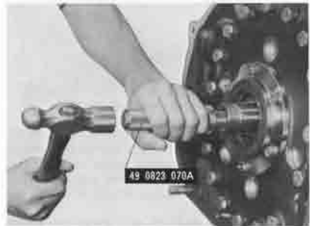
Fig. 1-60 Installing roller bearing
