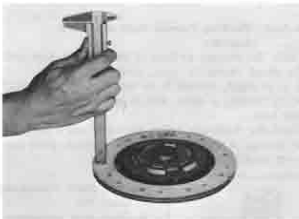
Fig. 6-10 Checking clutch disc for wear
