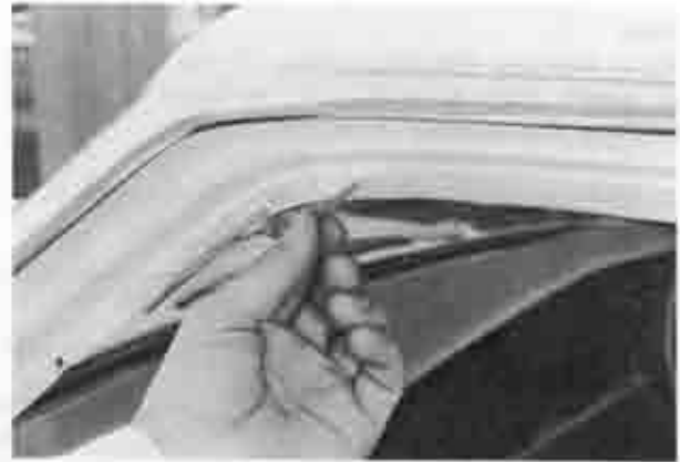
Fig. 14-91 Tearing of ceiling cemented surface
