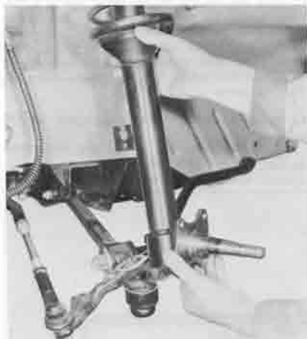
Fig. 13-3 Removing front shock absorber
