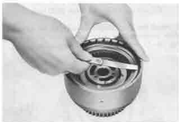
Fig. 7B-25 Measuring clearance
