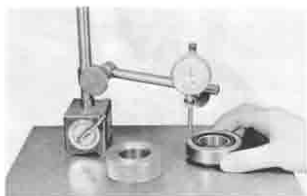
Fig. 9-25 Measuring bearing height
