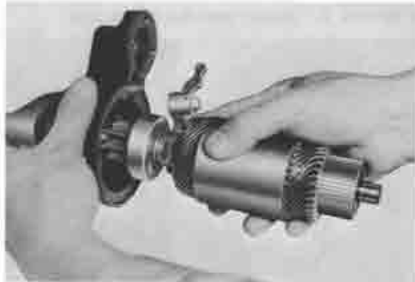
Fig. 5-36 Removing armature assembly
