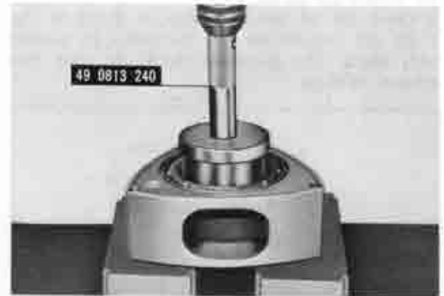
Fig. 1-43 Installing rotor bearing
