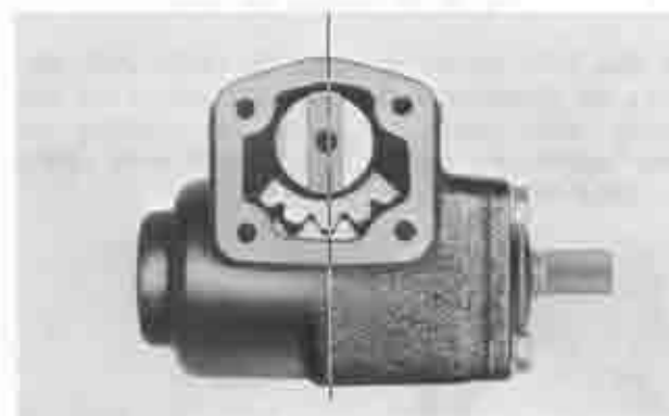
Fig. 10-12 Position of sector gear and worm gear
