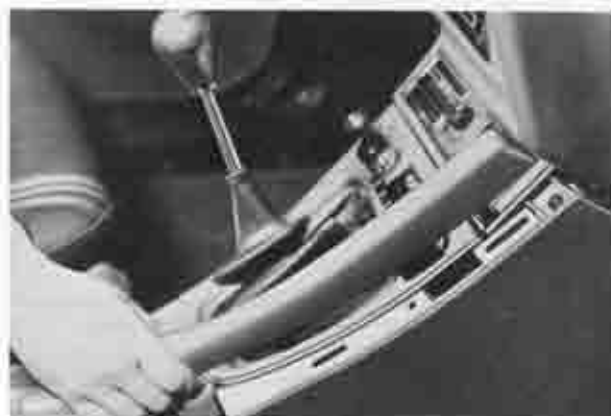
Fig. 14-97 Removing console pad
