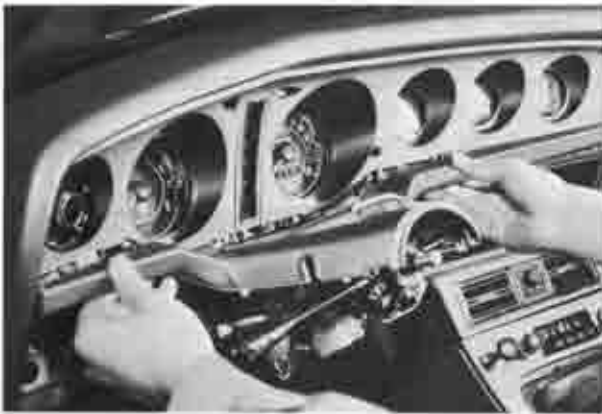
Fig. 15-17 Removing column cover upper
