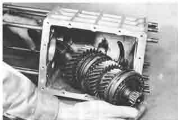
Fig. 7C-49 Installing main shaft and gears assembly
