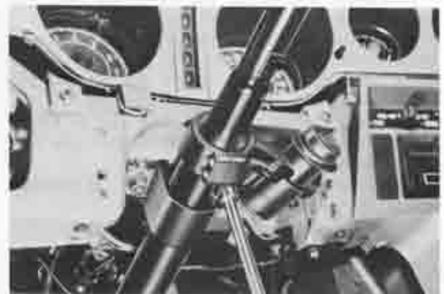
Fig. 10-22 Removing column shaft clamp
