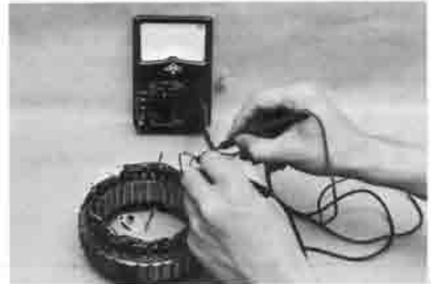
Fig. 5-20 Checking stator coil for open
