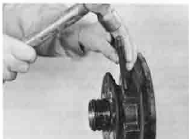
Fig. 12-7 Applying identification marks
