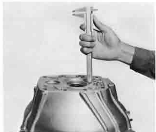
Fig. 7-38 Measuring bearing bore depth
