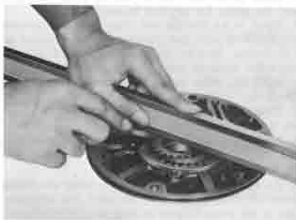
Fig. 7B-40 Measuring clearance (1)
