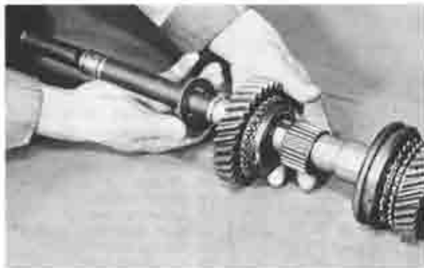
Fig. 7C-48 Installing first gear
