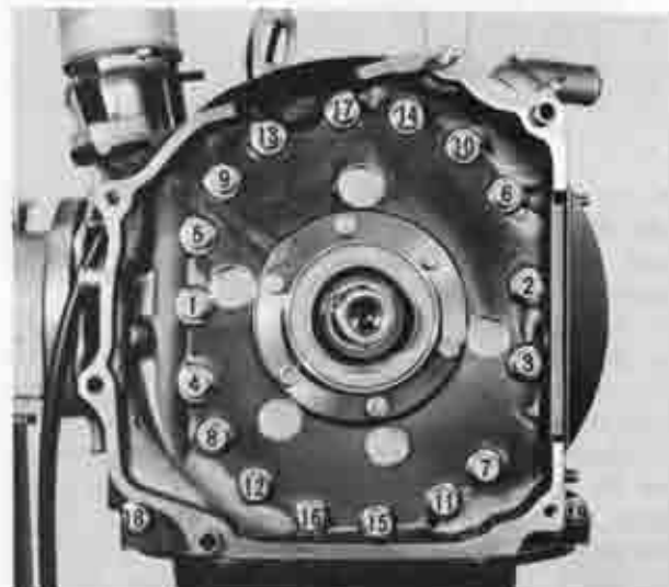
Fig. 1-79 Tension bolt tightening order
