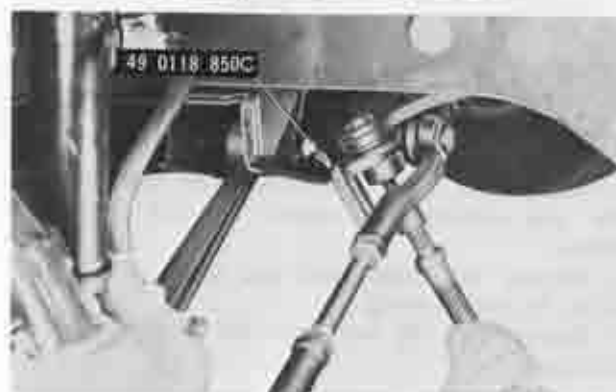
Fig. 10-2 Disconnecting center link
