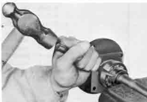
Fig. 9-4 Cutting bearing retaining collar
