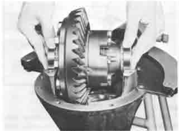
Fig. 9-12 Removing differential assembly
