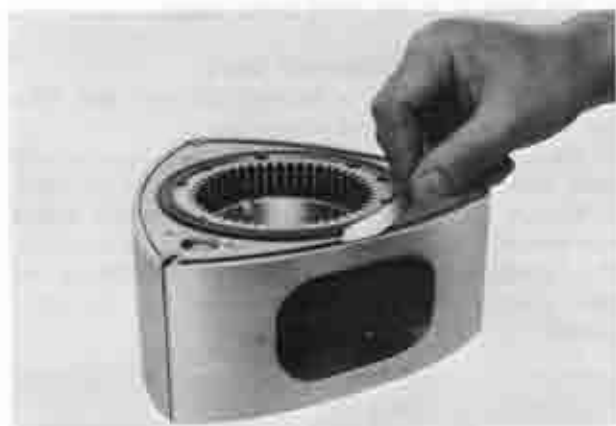
Fig. 1-51 Checking side seal gap
