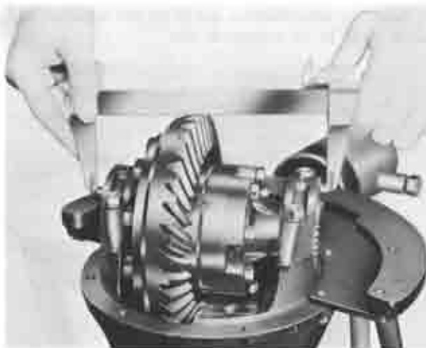
Fig. 9-35 Adjusting bearing preload (case spread)
