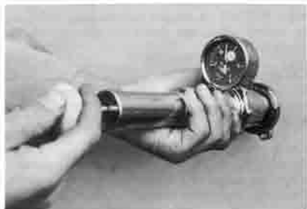
Fig. 3-7 Checking expansion tank cap
