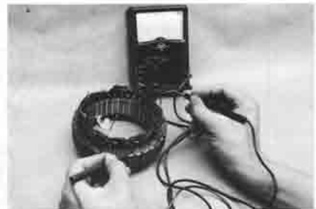
Fig. 5-21 Checking stator coil for ground
