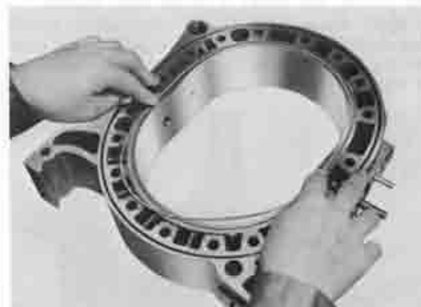
Fig. 1-70 Installing sealing rubber
