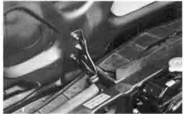
Fig. 14-2 Removing hinge attaching bolts
