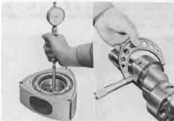
Fig. 1-41 Checking rotor bearing clearance
