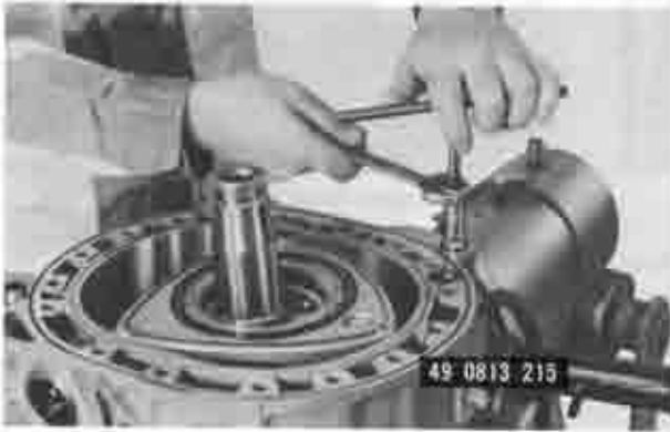
Fig. 1-20 Removing tubular dowel
