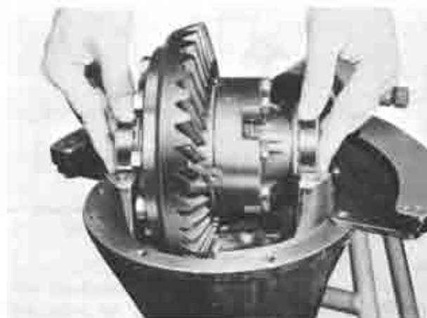
Fig. 9-12 Removing differential assembly
