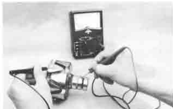
Fig. 5-21 Checking rotor for ground
