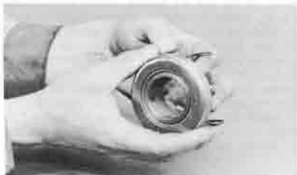
Fig. 6-5 Checking release bearing
