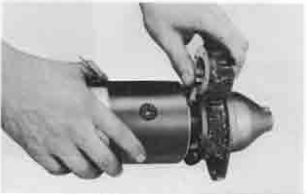
Fig. 5-33 Removing yoke assembly
