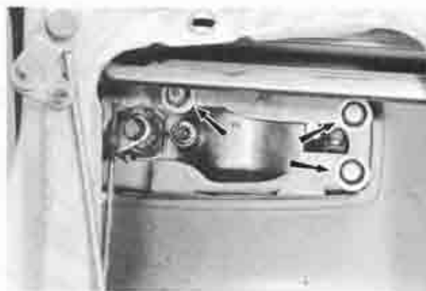
Fig. 14-55 Removing outer handle attaching bolts
