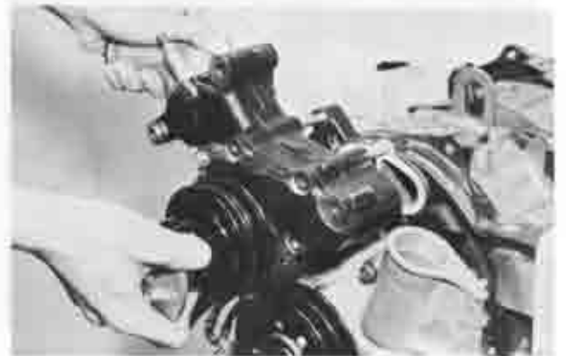
Fig. 1-88 Installing water pump
