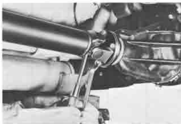
Fig. 7A-6 Removing propellar shaft
