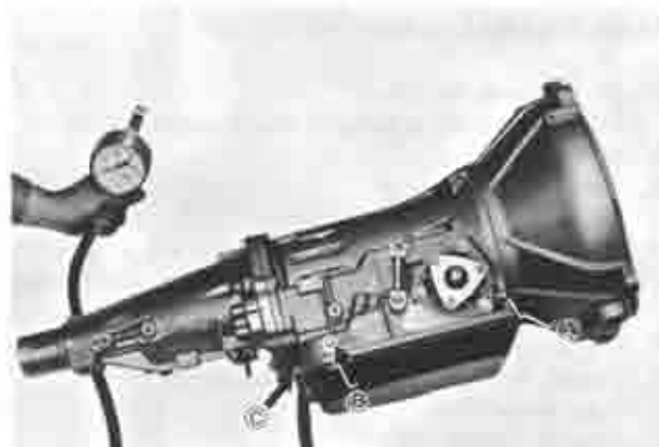
Fig. 7A-5 Oil pressure test
