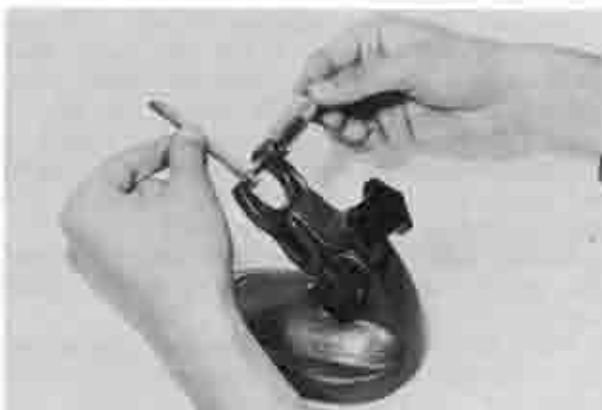
Fig. 1-43 Checking apex seal
