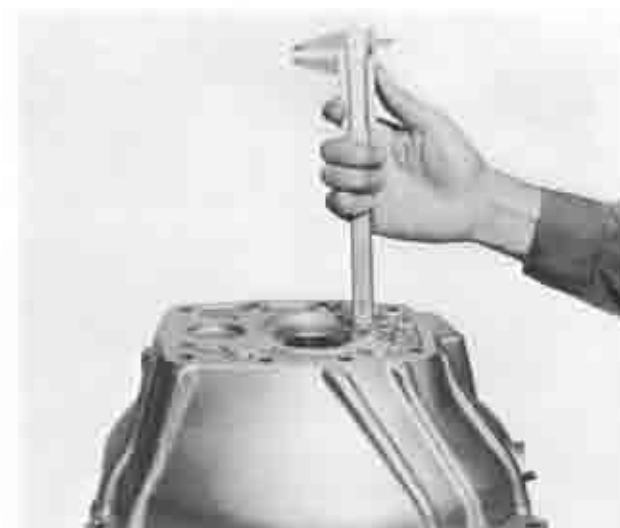
Fig. 7-38 Measuring bearing bore depth
