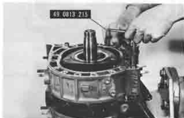
Fig. 1-20 Removing tubular dowel
