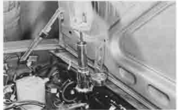
Fig. 3-4 Checking coolant leakage
