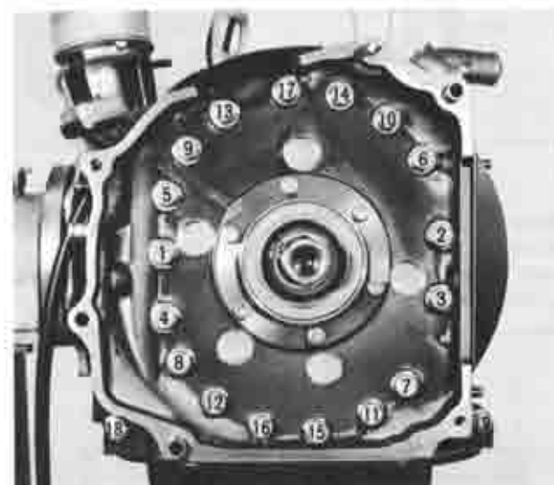
Fig. 1-75 Tension bolt tightening order
