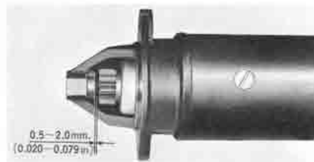
Fig. 5-43 Checking pinion position
