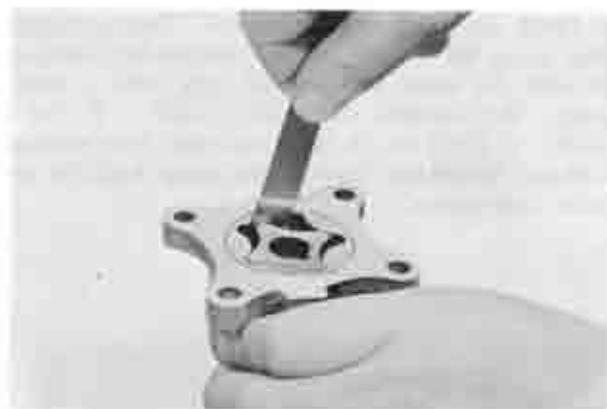
Fig. 2-3 Checking rotor clearance
