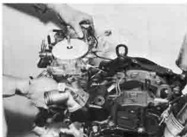
Fig. 1-92 Installing intake manifold assembly
