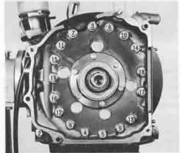
Fig. 1-17 Tension bolts loosening order
