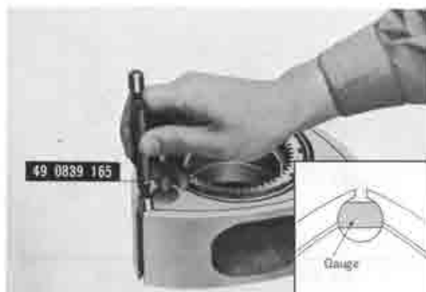
Fig. 1-50 Checking corner seal groove
