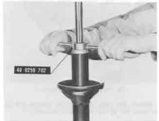
Fig. 13-26 Tightening cap nut temporarily
