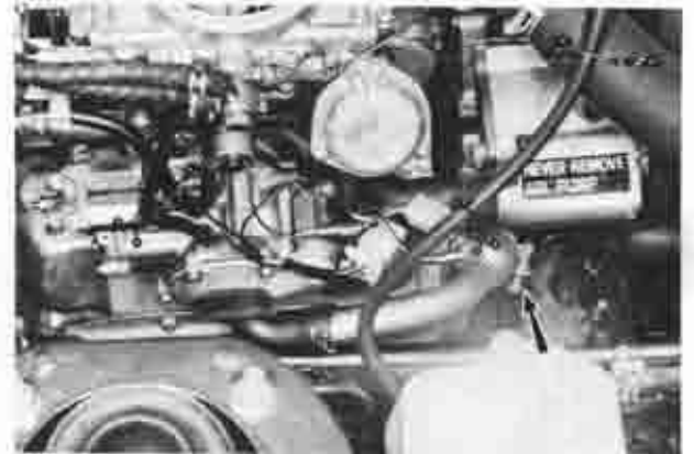
Fig. 1A-8 Removing air pipe
