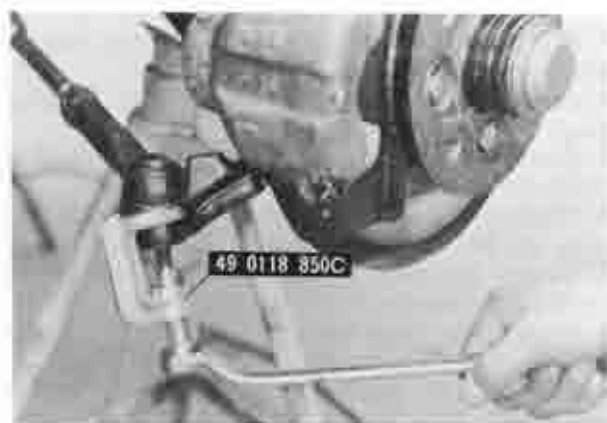
Fig. 10-25 Disconnecting tie-rod end
