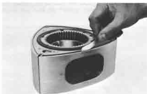
Fig. 1-48 Checking side seal gap
