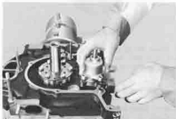
Fig. 2-2 Removing oil pump
