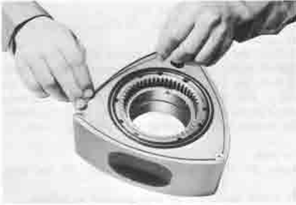
Fig. 1-61 Installing side seal
