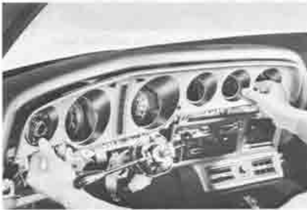
Fig. 15-18 Removing meter cover
