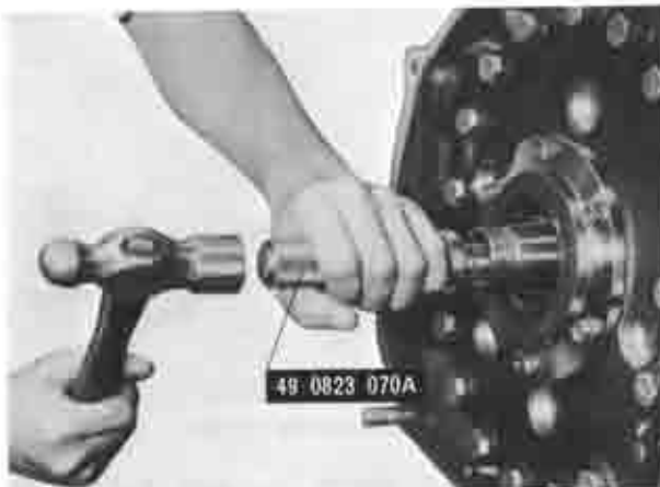
Fig. 1-55 Installing roller bearing
