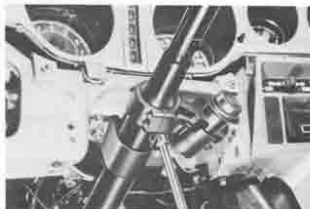
Fig. 10-22 Removing column shaft clamp
