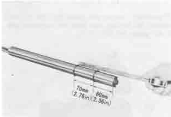
Fig. 13-23 Installing oil stop rings
