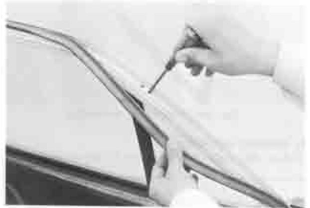
Fig. 14-68 Removing upper end attaching screws
