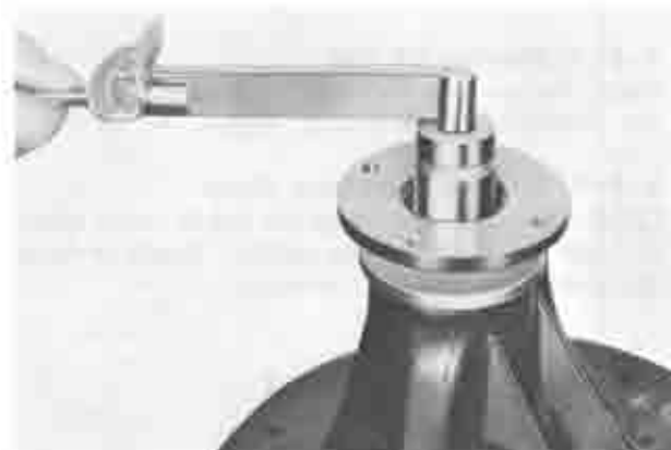
Fig. 9-26 Checking pinion bearing preload
