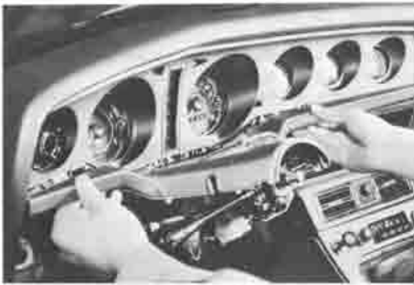
Fig. 15-17 Removing column cover upper
