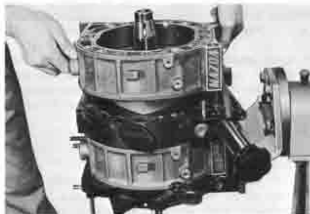
Fig. 1-73 Installing rear rotor housing
