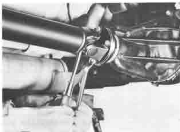
Fig. 8-1 Removing propeller shaft attaching bolts
