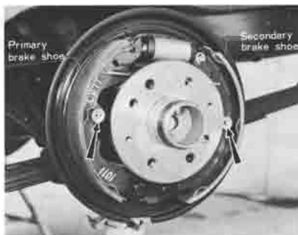
Fig. 11-39 Removing shoe hold-down spring
