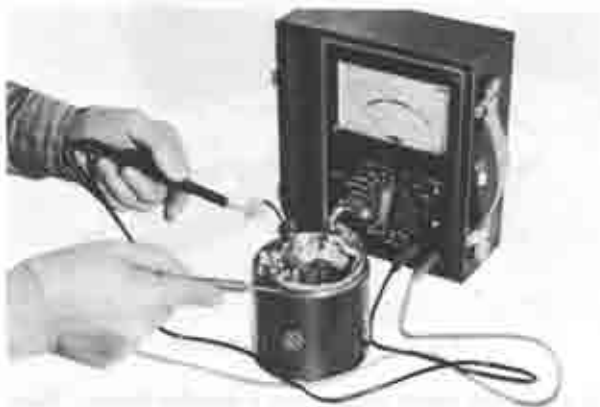
Fig. 5-39 Checking field coil for ground
