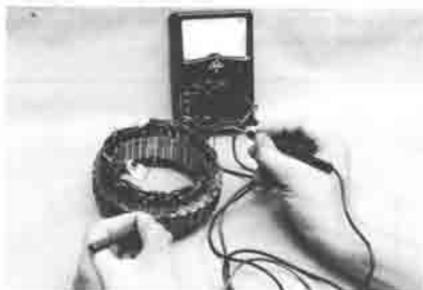
Fig. 5-19 Checking stator coil for ground
