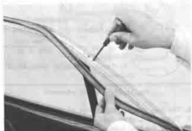
Fig. 14-66 Removing upper end attaching screws
