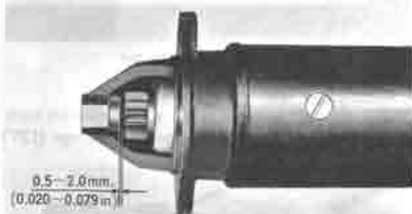
Fig. 5-31 Checking pinion position
