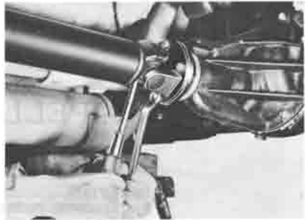
Fig. 8-1 Removing propeller shaft attaching bolts
