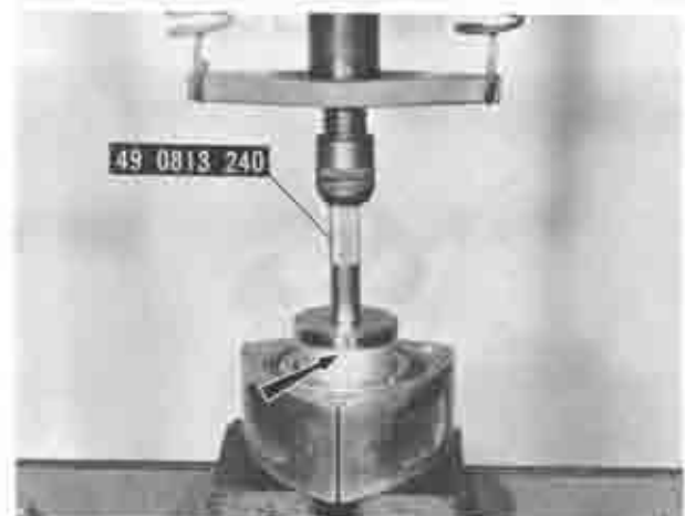
Fig. 1-40 Installing rotor bearing
