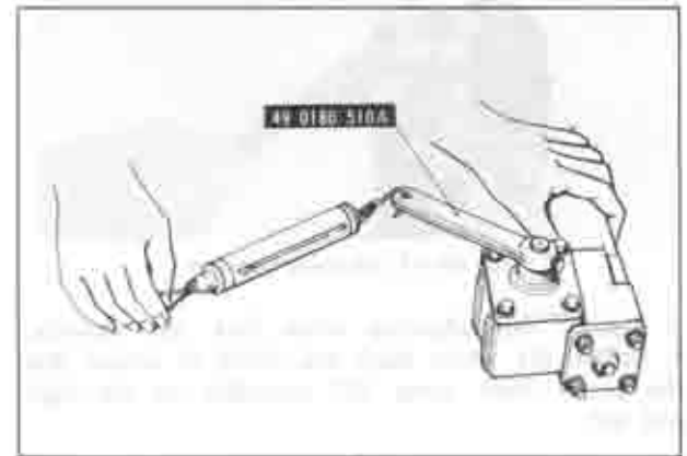
Fig. 10-16 Checking bearing preload
