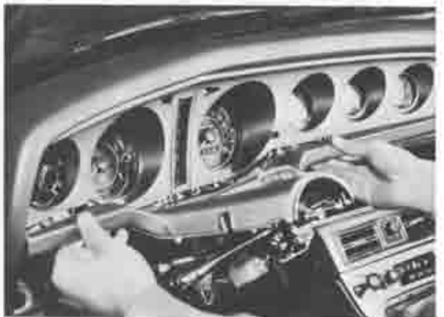
Fig. 15-18 Removing column cover upper
