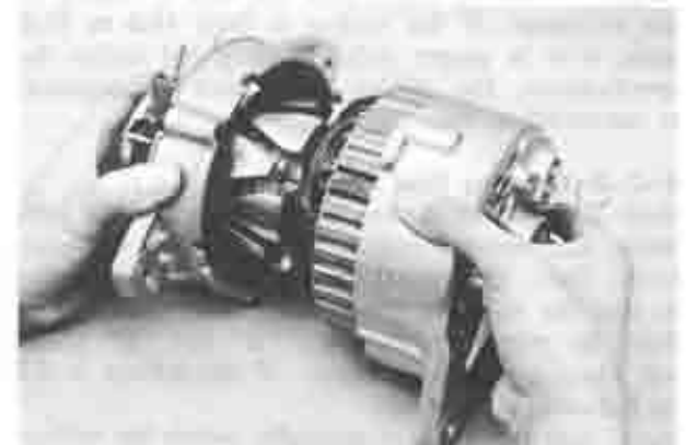
Fig. 5-12 Installing rotor assembly
