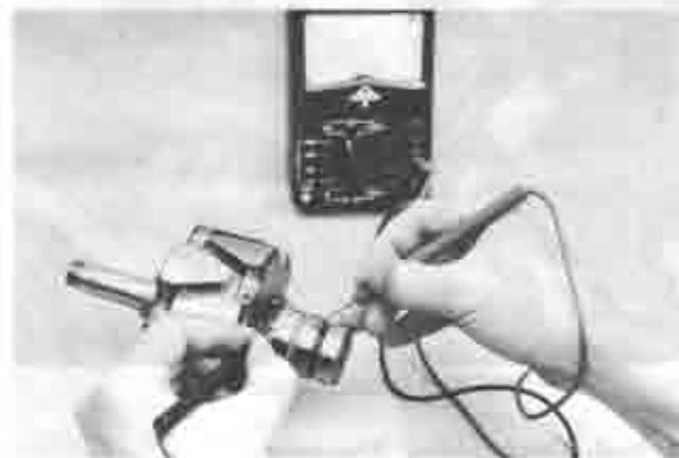
Fig. 5-8 Checking rotor for open
