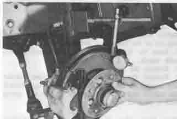
Fig. 11-34 Checking brake disc run-out
