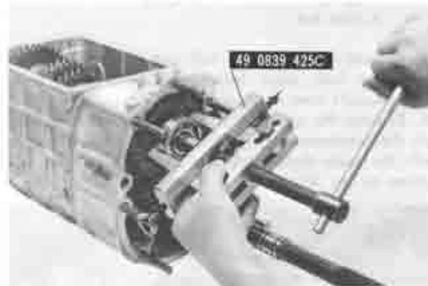
Fig. 7A-14 Removing counter shaft rear bearing
