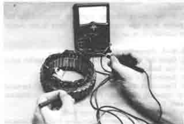
Fig. 5-7 Checking stator coil for ground
