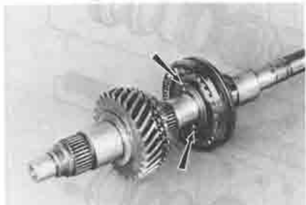
Fig. 7A-45 Installing clutch hub assembly (1st & 2nd)
