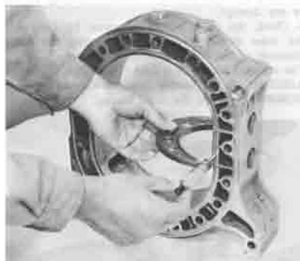
Fig. 1-35 Checking rotor housing width
