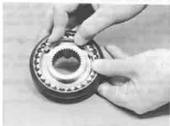
Fig. 7-16 Installing synchronizer key spring
