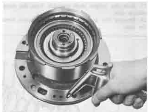
Fig. 7B-28 Testing front clutch
