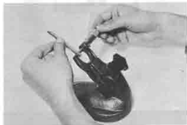
Fig. 1-43 Checking apex seal height
