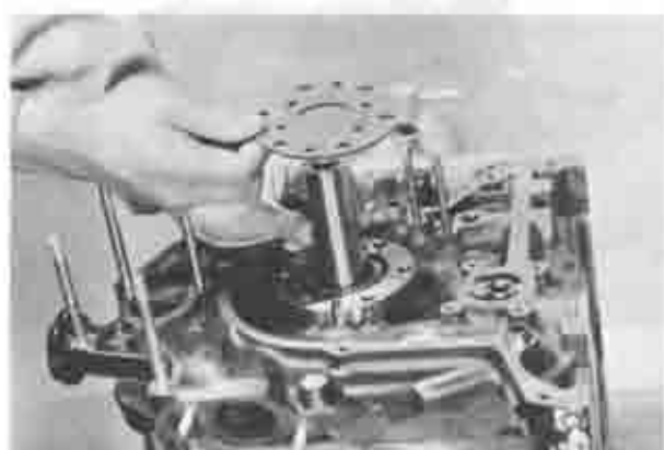
Fig. 1-78 Installing bearing housing
