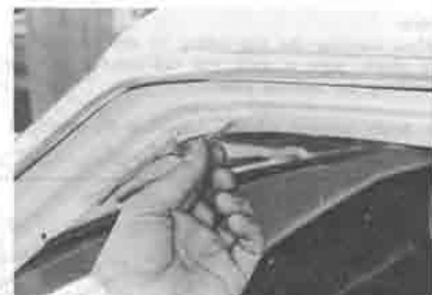
Fig. 14-88 Tearing of ceiling cemented surface
