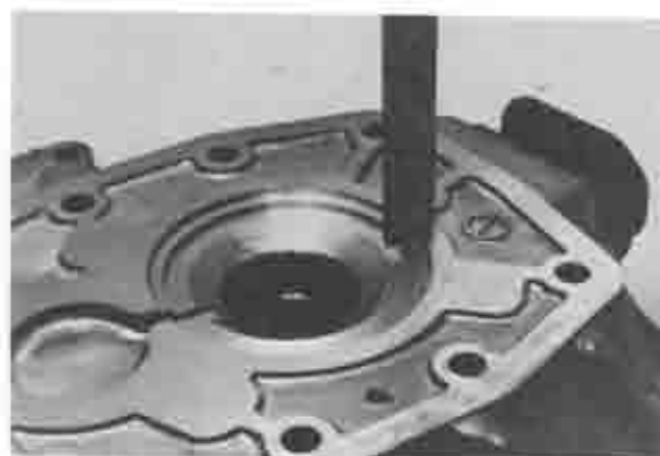
Fig. 7A-74 Measuring bearing bore depth
