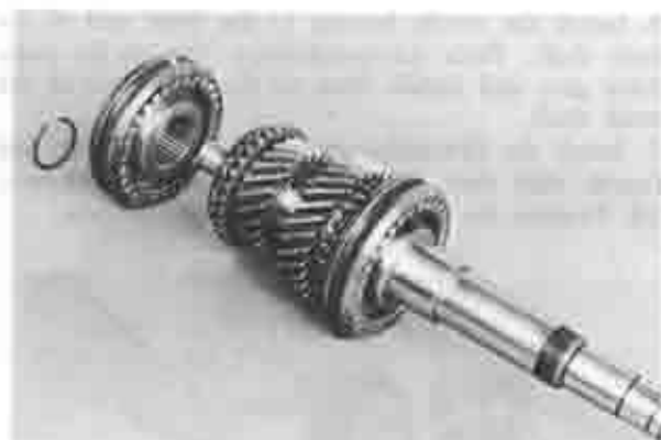
Fig. 7-18 Installing clutch assembly (3rd & 4th)
