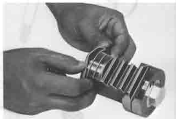
Fig. 10A-17 Installing Teflon ring
