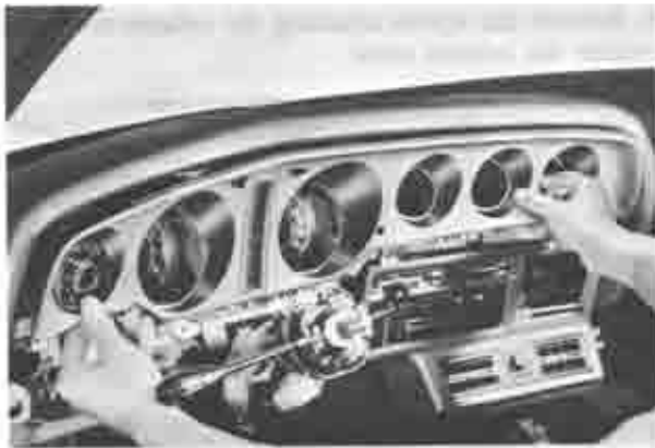
Fig. 15-19 Removing meter cover
