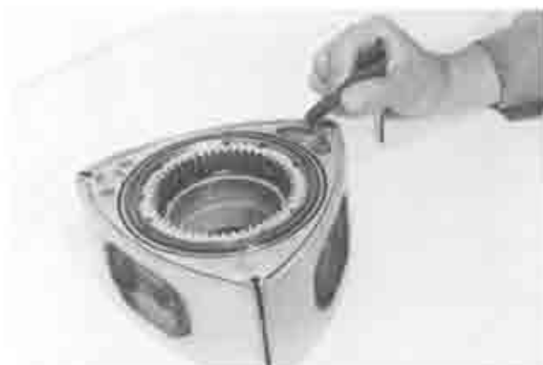
Fig. 1-48 Checking seal clearance
