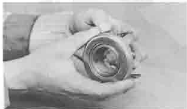
Fig. 6-5 Checking release bearing
