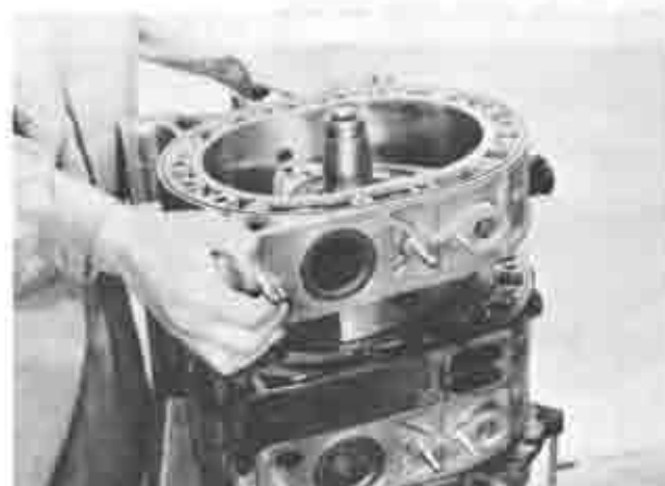
Fig. 1-70 Installing rear rotor housing
