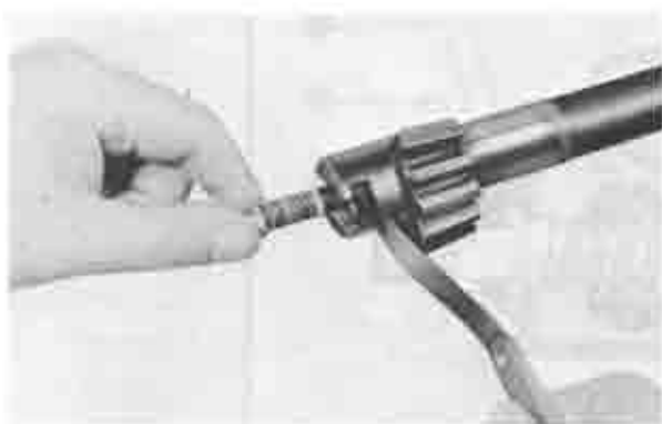
Fig. 10-10 Checking end clearance
