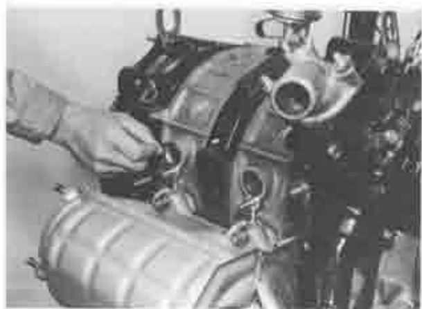
Fig. 1-93 Installing "O" ring
