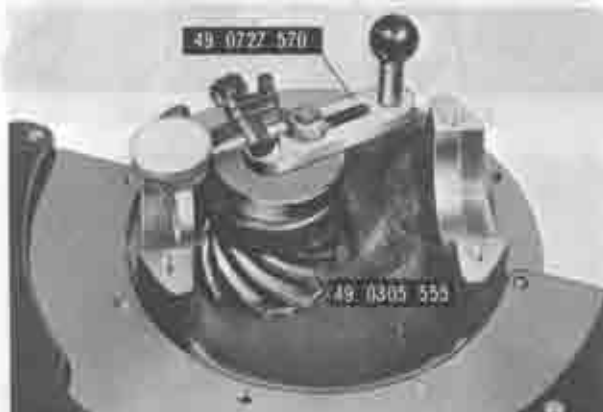
Fig. 9-22 Measuring pinion height
