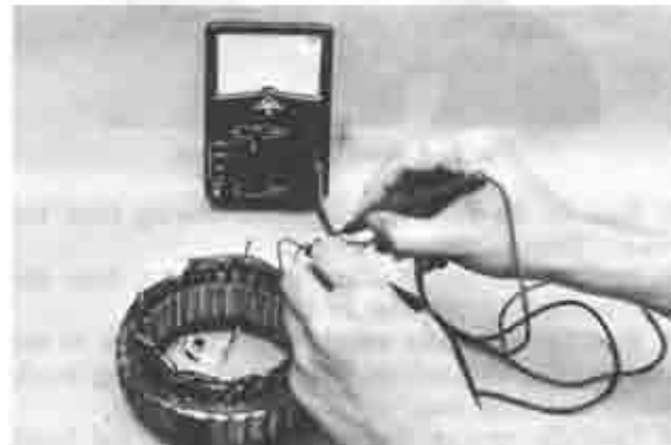
Fig. 5-5 Checking stator coil for open
