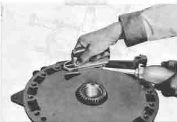
Fig. 1-24 Cleaning front housing
