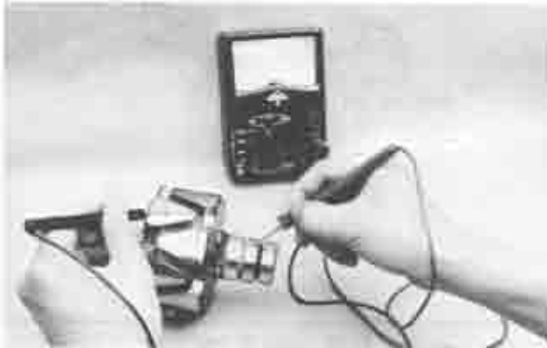
Fig. 5-9 Checking rotor for ground
