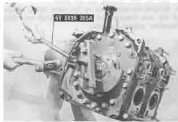
Fig. 1-13 Removing counter weight
