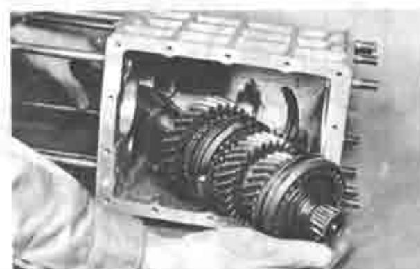
Fig. 7A-49 Installing main shaft and gear assembly
