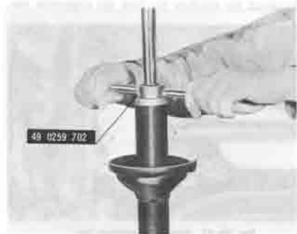
Fig. 13-10 Tightening cap nut temporarily
