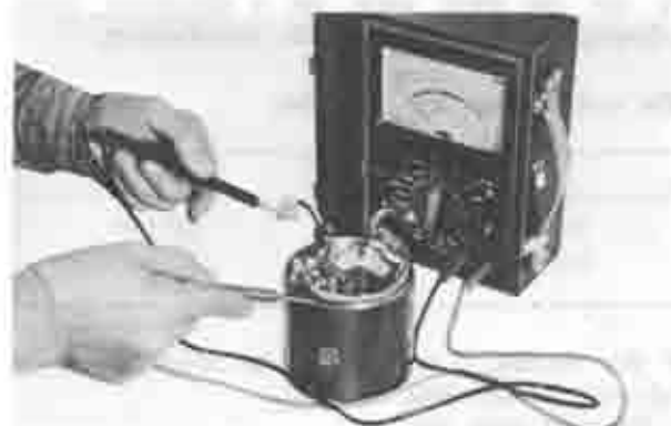
Fig. 5-27 Checking field coil for ground
