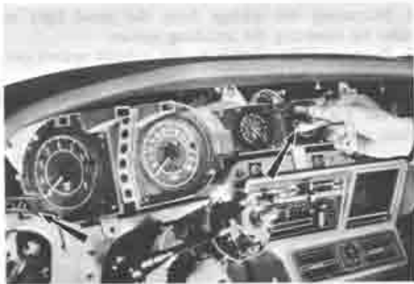
Fig. 15-20 Removing wiring connector
