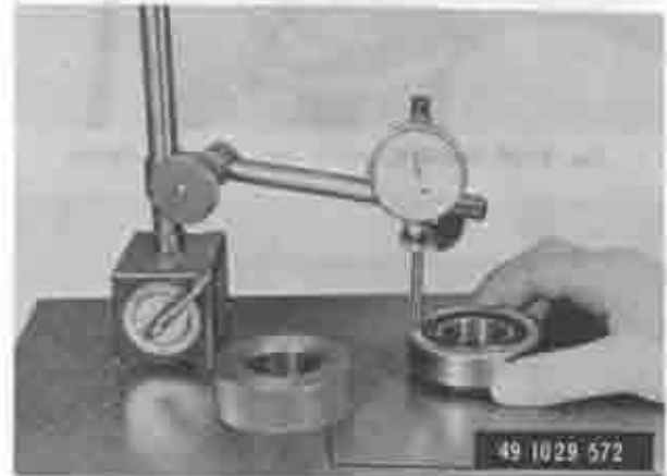
Fig. 9-23 Measuring bearing height
