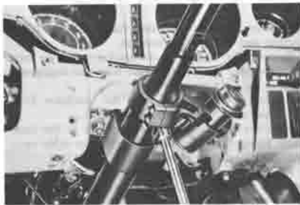
Fig. 14-98 Removing steering shaft bracket
