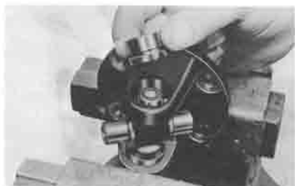
Fig. 8-16 Installing bearing cap assembly
