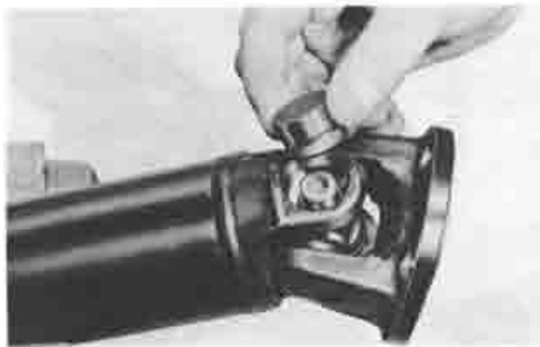
Fig. 8-19 Installing bearing cup
