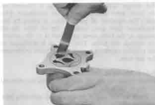
Fig. 2-10 Checking outer rotor clearance
