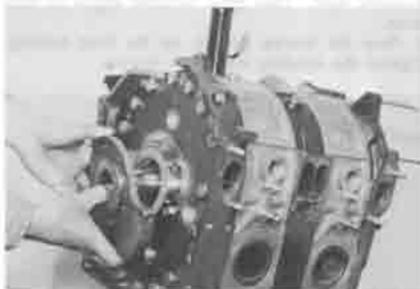
Fig. 1-75 Installing counter weight
