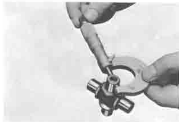
Fig. 8-15 Measuring spider diameter
