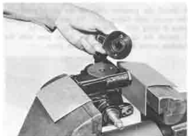
Fig. 10A-43 Installing suction line connector
