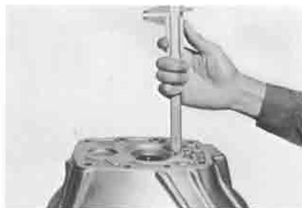
Fig. 7-35 Measuring bearing bore depth
