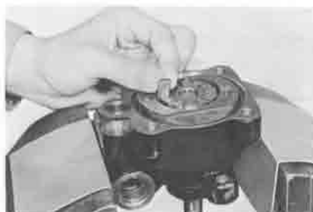
Fig. 10A-38 Installing vanes
