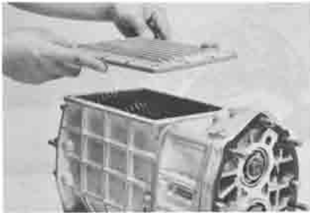
Fig. 7A-10 Removing under cover
