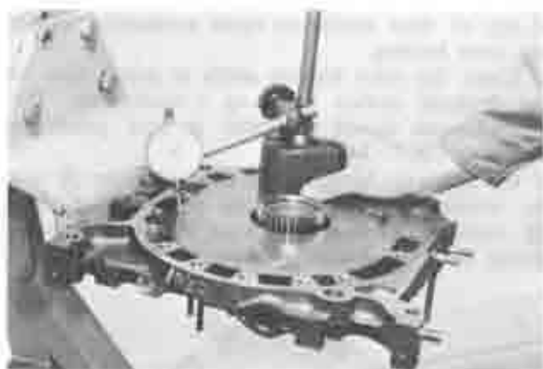
Fig. 1-27 Checking housing for wear
