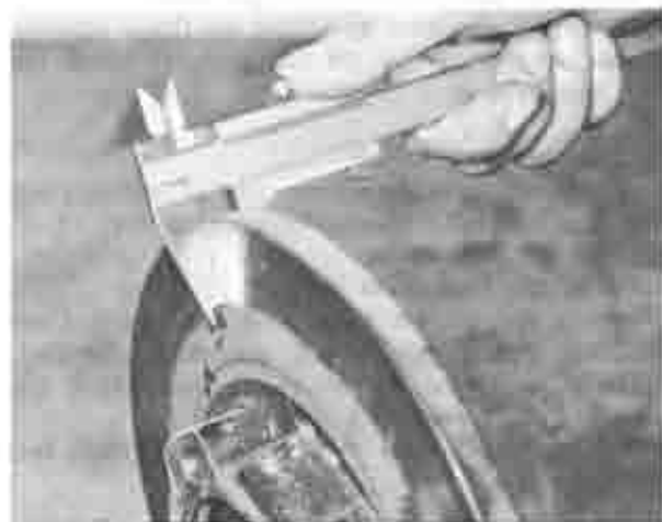
Fig. 11-36 Checking brake disc thickness
