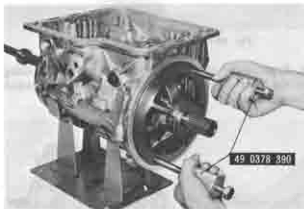
Fig. 7B-18 Removing oil pump
