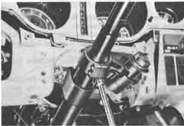
Fig. 14-98 Removing steering shaft bracket
