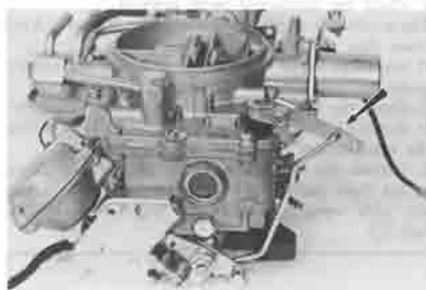
Fig. 4-23 Specified hole of accel. pump lever
