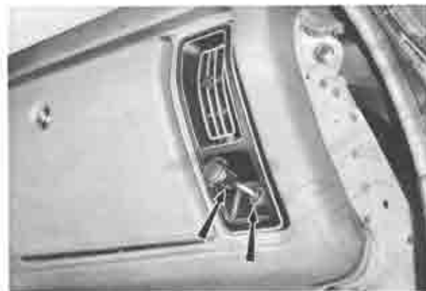
Fig. 14-99 Removing ventilator knob
