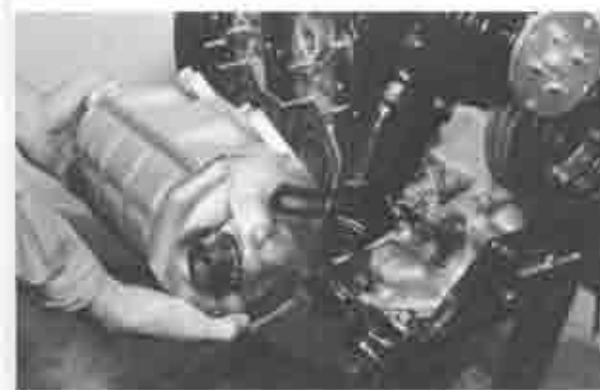
Fig. 1-4 Removing thermal reactor
