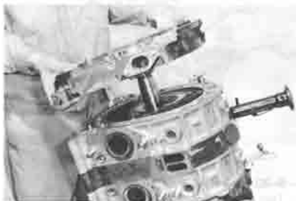
Fig. 1-16 Removing rear housing
