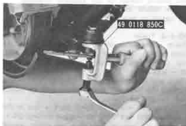
Fig. 10-22 Disconnecting tie-rod end
