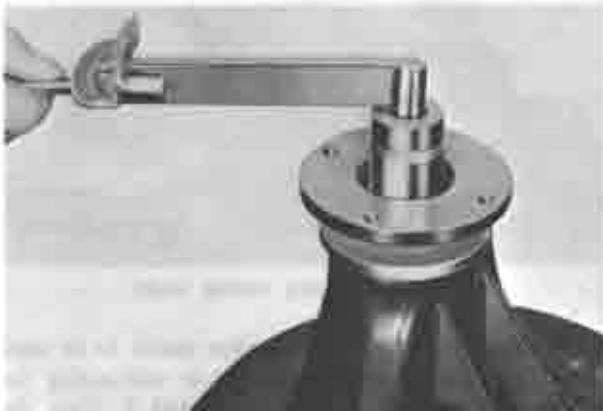
Fig. 9-25 Checking pinion bearing preload
