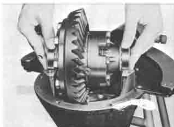
Fig. 9-12 Removing differential assembly
