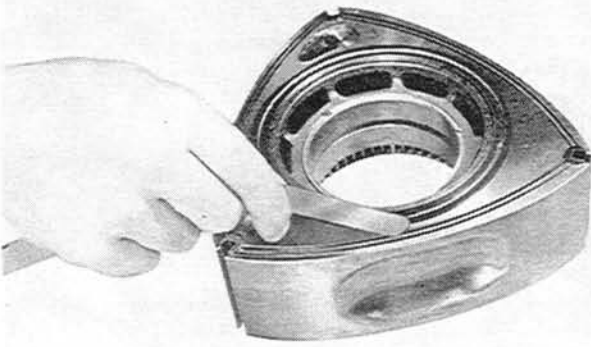
Fig. 1-63 Checking side seal gap
