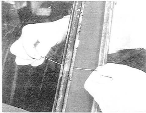
Fig. 14-4 Piercing of piano wire
