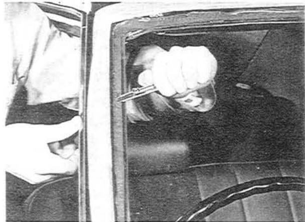
Fig. 14-7 Cutting of sealant
