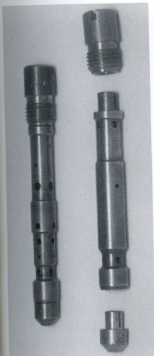
Dellorto main jet, emulsion tube and an emulsion tube holder dismantled (right) and assembled (left). Note that the air correction hole is part of the holder.
