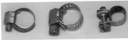
A range of small clamps suitable for use on fuel lines (pipes). Use clamps of the correct size.
