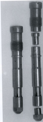
Weber main jet, emulsion tube, air corrector jet and an emulsion tube holder dismantled (right) and assembled (left).
