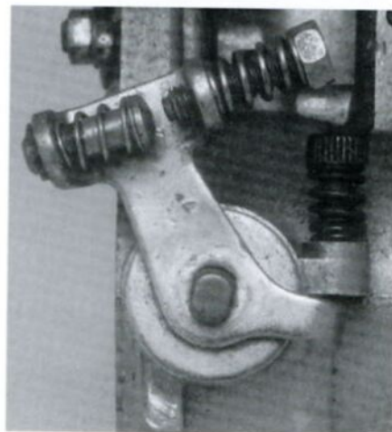
Weber linked-type throttle arm positioned on the throttle spindle. Note that it must be a tight fit.
