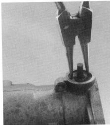
A throttle spindle dust cap being removed from a Weber using circlip pliers (after the body has been heated).
