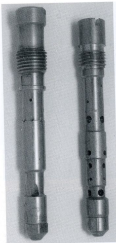
Left - Comparison of Weber (left) and Dellorto (right) main jets, emulsion tubes and holders.
