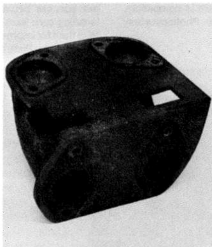
Experimental phenolic intake manifold was devised by Rick Engman and used in GTU competition. In addition to isolating carburetor from heat, manifold incorporates D-shaped runners that extended power range.
