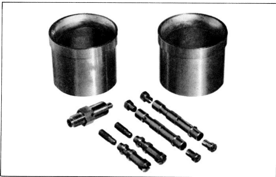
In addition to tuning 48 IDA Weber, it can be enlarged to 51mm. When done, new venturis are required as are new air/fuel calibrations. Air jets, fuel jets, emulsion tubes and venturis are all readily available through Weber specialists. Photo courtesy Racing Beat.
