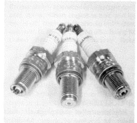
Sparkplug choice depends on application and personal preference. For street use, a multi-electrode plug such as one at left is recommended. Racing plugs are typically of the surface-gap (center) or standard single-electrode variety.
