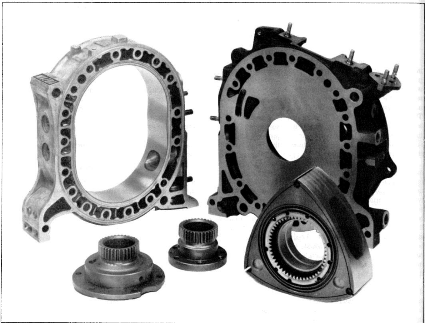
In high-performance rotary engines, rotor-to-housing clearance must be set to compensate for variances in stationary-gear indexing. Components are from a Racing Beat bridge-ported engine. Water-jacket modifications (see Chapter 8) are visible on rotor housing.
