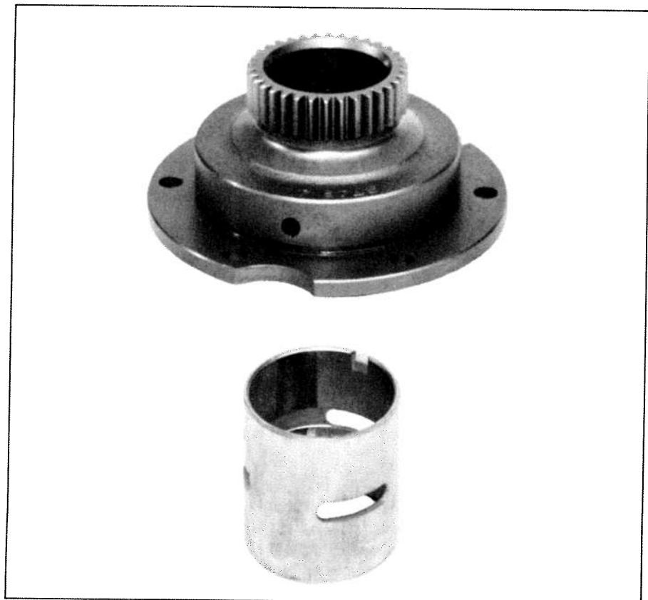
Special three-window bearing is used in race engines to provide improved oil circulation between bearing and eccentric shaft. In order to be effective, three-window bearings must be used with a modified stationary gear.
