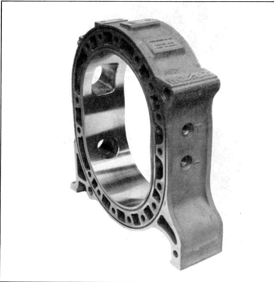
Rotor housings with peripheral intake ports are found only in race engines. Port timing is too radical for an engine with an exhaust system that includes a muffler of any consequence.
