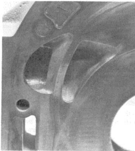
As can be seen, outside wall of port encroaches into area normally occupied by red rubber inner seal that contains coolant flowing through water jacket.
