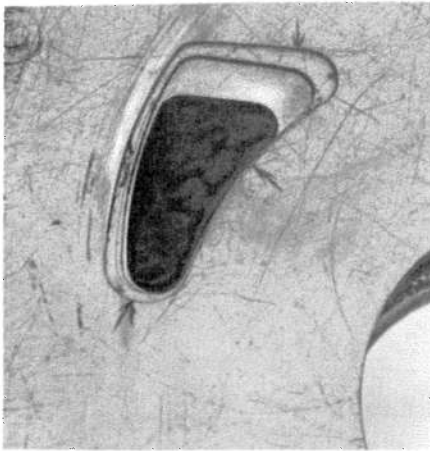
Porting templates illustrate extent to which port shapes are changed for high-performance operation. Due to path traveled by rotor, left port-wall position determines opening timing. Rounded apex at upper right controls closing.
