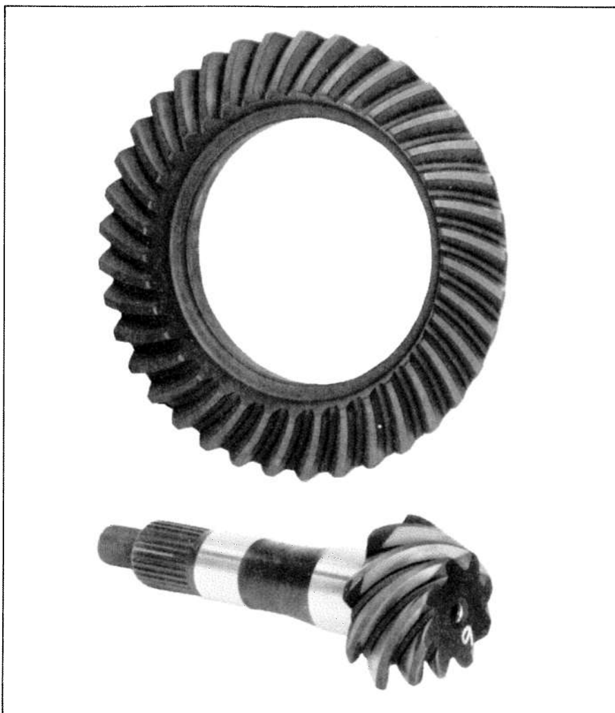
Rear-axle ratio, as determined by ring and pinion gears, has a significant affect on both performance and fuel economy. When making extensive engine modifications, it may be necessary to switch to a lower gear ratio (higher numerical ratio) to compensate for less low-speed torque. Photo courtesy Racing Beat.
