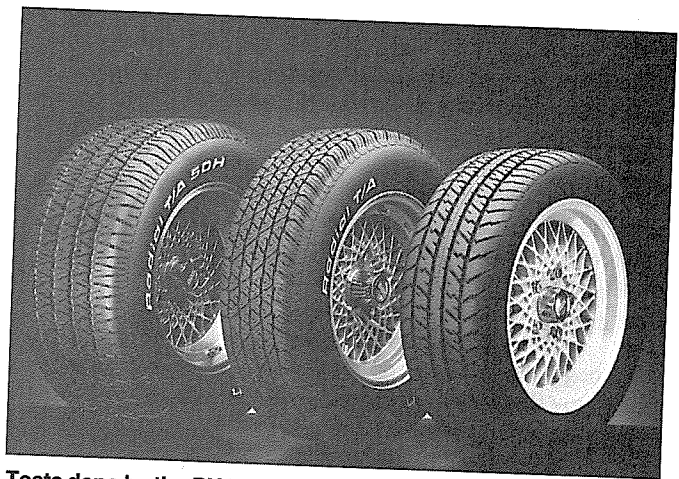
Tests done by the RX-7 Club of America have consistently shown the BFGoodrich Comp T/As (right) to rank at the top of the handling list. At left is the Euro-Radial T/A which offers a bit less cornering power, but at a considerably lower price. Standard Radial T/A is in the center.
