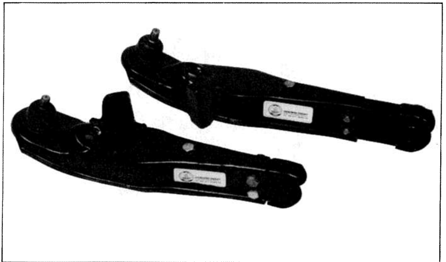
Adjustable front-suspension lower control arms for 1979—85 RX-7s from Racing Beat increases front-suspension camber-adjustment range. Note compressed and extended control-arm lengths. Photo courtesy Racing Beat.
