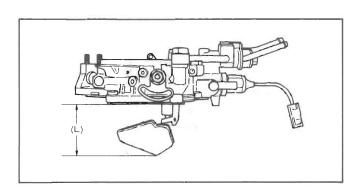
45. Install air horn on main body with two (longest) screws near fuel inlet.\*
