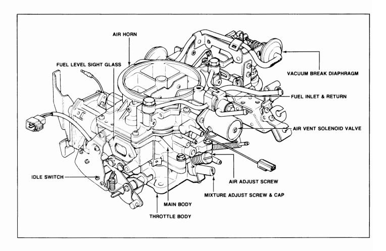
1979 – 1985 RX-7 vehicles came equipped with NIKKI 4-barrel carburetors. These carburetors are of a downdraft design and are equipped with semi-automatic chokes. Various solenoids are installed for driveability and emissions. Some versions feature a special Sub-Zero system which injects a mixture of anti-freeze into the carburetor for easier starting in cold climates. Also featured is a system of oil injection through the carburetor.
