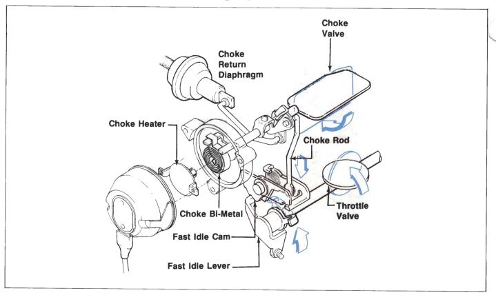
While the choke is on, a fast-idle system is also used to help prevent stalling and to provide a smooth idle. The fast-idle is operated by the choke linkage and is used to increase idle speed.
