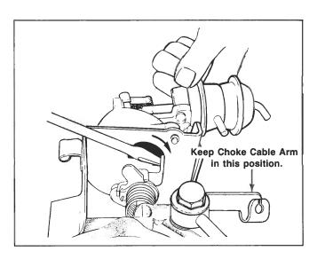
If necessary, use a screwdriver to assist in aligning the choke shaft lever and the bi-metal spring, but be careful not to damage the bi-metal or heater element by doing so.
