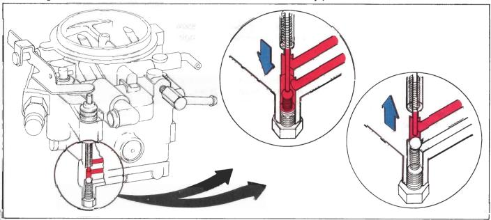
To prevent the above condition, a fuel cut valve has been installed in the secondary main fuel passage. The fuel cut valve is operated by the accelerator pump lever and cuts the secondary fuel supply when the throttle is closed.
