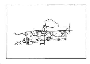
This clearance should be 16  $\pm$  0.5 mm (0.63  $\pm$  0.02 in). If the clearance is not within specifications, bend the float seat lip until the proper clearance is obtained.
