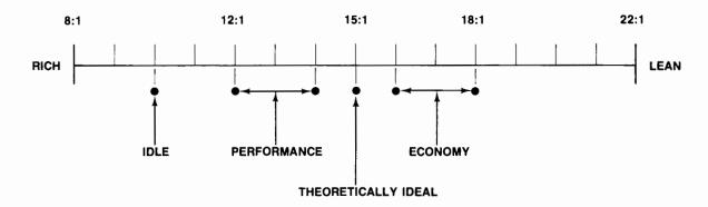
When we talk about air/fuel mixture or ratio we are talking about the number of parts of air compared to one part fuel, measured by weight.
